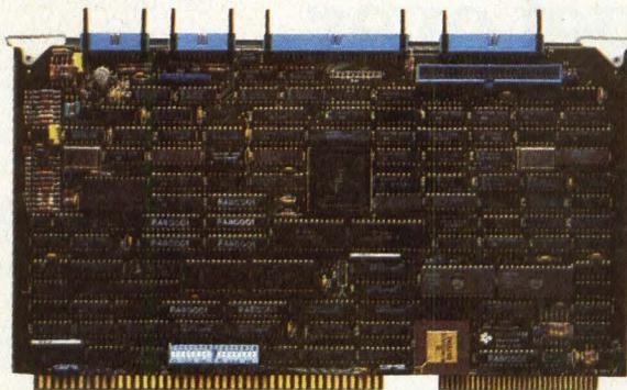
for the very first time on a controller, Storer has an *on-board* 68000 CPU.
