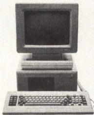
Monitor conveniently tilts and swivels. Pedestal height is proper. Green, amber or color non-glare monitors all meet toughest ergonomic standards. Three position keyboard is smooth as silk. Meets European ergonomic standards. Smart alpha and numeric shift lamps don't get fooled when software changes keyboard state. Dimpled F and J keys indicate home keys.
