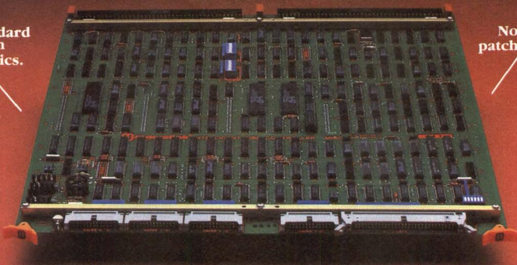
Only our Macrolink Intelligent Disk Controller (MIDC) offers full software and disk pack compatibility with the P-E IDC system. Using such advanced features as on-board ECC logic and micro-coded bit slice technology, MIDC corrects errors of up to 11 bits without operating system overhead. And when you plug this single-board controller into your Series 3200 CPU, you
