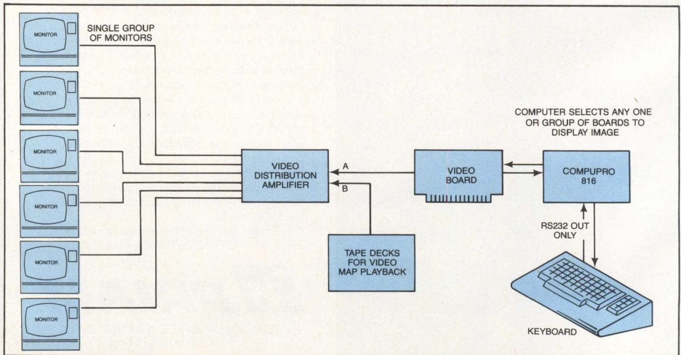
Dividing the set's 120 monitors into 20 groups of six, each controlled by a single S-100 bus video board, enabled 20 different
