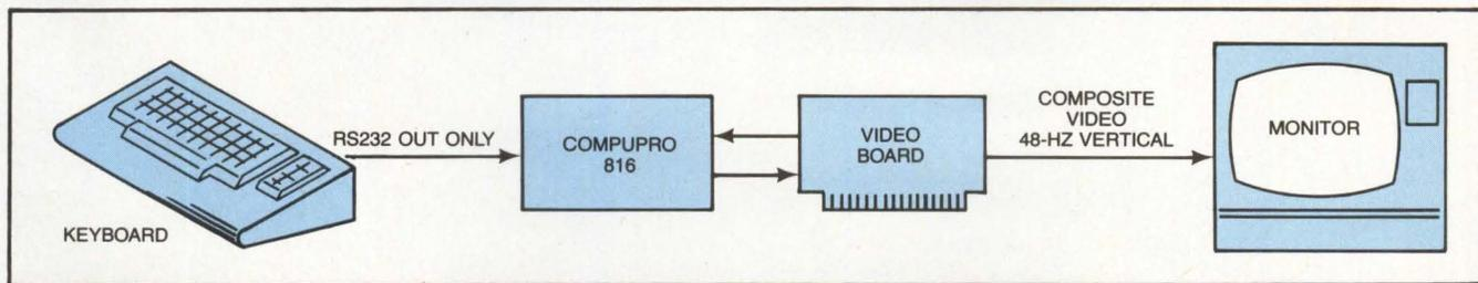
**Echo-replacement software** automatically displayed a predetermined message on the monitor, one character at a time, no matter what key the actor hit. Software also replaced the input signal with a
