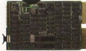
2. Q-BUS RX02 COMPATIBLE 5 1/4" FLOPPY DISK CONTROLLER-MXV22M.
