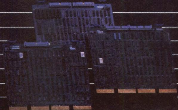
1/2" TAPE—CONTROLLER/COUPLER PERTEC I/O
