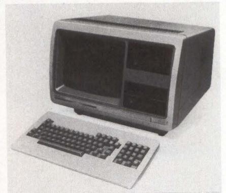
vendor's proprietary operating system and UNIX. \$7,995, including 512K bytes of memory, the CRT, a keyboard, a 10M-byte Winchester disk drive, a 1M-byte floppy disk drive, the MCS operating system and a programming language. **Wicat Systems**, P.O. Box 539, 1875 S. State, Orem, Utah 84057, (801) 224-6400. **Circle No 306**
