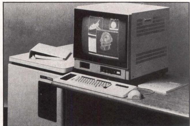
**Apollo's DN 660 computational node** aims at complex solids-modeling and image-analysis applications. The color display incorporates 2M bytes of dedicated RAM providing 1,024-by-1,024-pixel resolution. All Apollo nodes are network-compatible and can concurrently run UNIX and Apollo's Aegis operating system.
