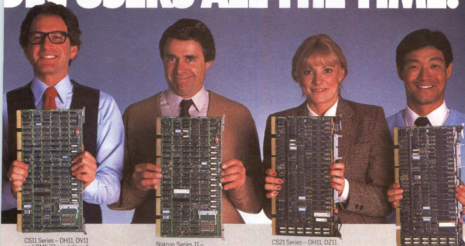
CS11 Series – DH11, DV11 and DMF-32 emulations for PDP-11 and VAX-11 CPUs. Handles 8 to 64 asynchronous lines.
