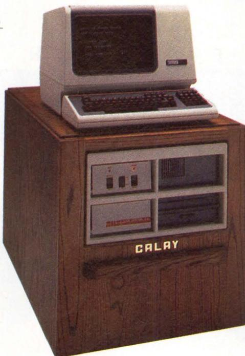
your existing CAD environment the Calay RPR-300 Router and feed it the data from your REDAC or APPLICON. After a short time of the fully automatic routing process, you get the complete data of a routed PC board, which is fed back to your original CAD system for output documentation purposes.
