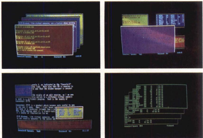
console number (0, 1, 2, 3). PR and PC are the row and column coordinates of the upper-left corner of each window, and NR and NC are the number of rows and columns. PC and PR are staggered to allow for overlap. NR and NC are constant because all windows in this display are the same
