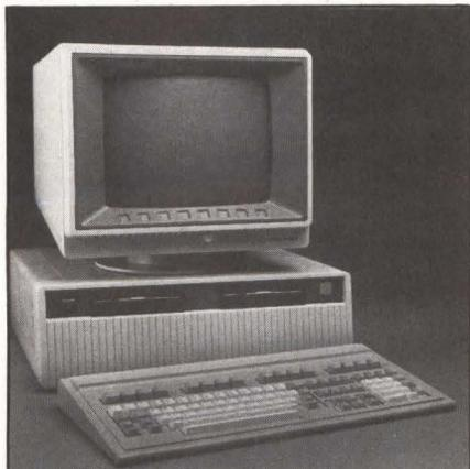
One of many products in Perkin-Elmer Corp.'s comeback strategy is the new 68000-based 7350 Professional Computer. The 7350 is designed as a standalone product or as a companion product integrated with P-E's Series 3200 supermini-computers. Applications written in C and FORTRAN can be ported between the 7350's UniPlus operating system and the OS/32 real-time operating system of the larger machines.
