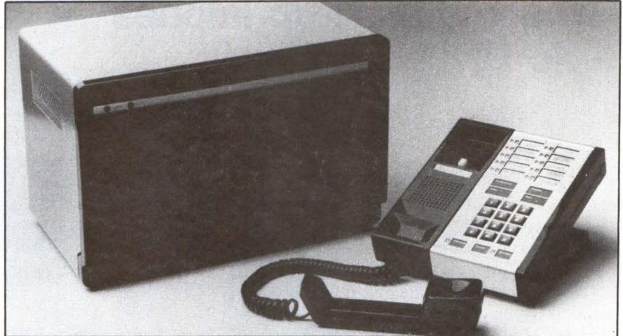
**The Merlin communications system is ATTIS' key system. It serves small business customers with as many as four lines and 10 telephones. The control unit is on the left, and the 10-button telephone is on the right (five- and 34-button sets are also available.)**
