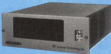
When used as a disc replacement, the high speed, non-rotating MegaRam provides the software compatibility of a disc with the performance of main memory. Ideal for swapping, scratch files, overlay storage, process control, telecommunications, graphics, data acquisition, array processing, etc.
