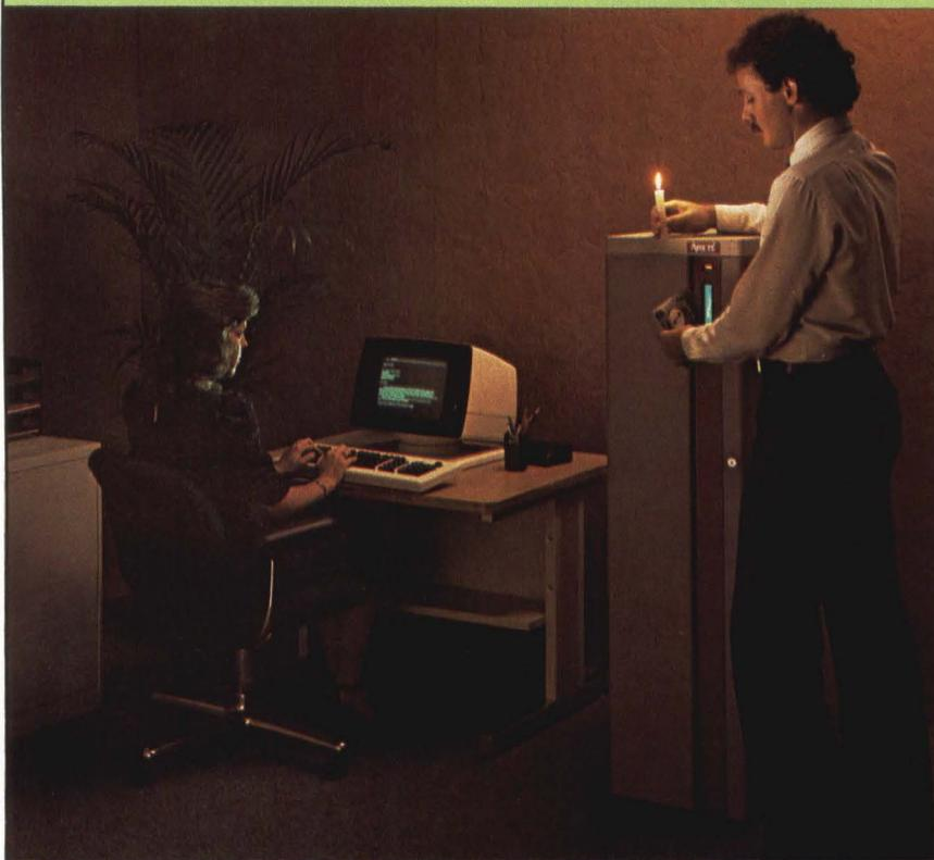
Arete Systems Corp.'s 32-bit fault-tolerant system provides eight hours of battery backup. When a power failure occurs, sensors immediately notify the CPU to switch to backup.
