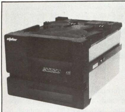
Cipher Data Products Inc.'s first entry with a group-code-recording (GCR) ½-inch tape drive is the CacheTape M990. The drive features 128K bytes of cache memory, a 450K-byte-per-second transfer rate and a 125-inch-per-second streaming speed.
