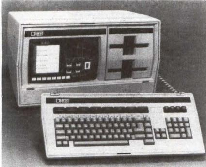
connection to the host or a printer. The model 1625 is host-compatible with the HP 3000. It has an application-specific keyboard and provides an HP terminal personality with block-mode capabilities. The model 1631 has a DEC VT100 terminal personality and complies with the ANSI X3.64 standard. \$3,995 each. Delivery is 60 days after receipt of order. **Direct Inc.**, 4201 Burton Dr., Santa Clara, Calif. 95051, (408) 980-1414. **Circle No 302**
