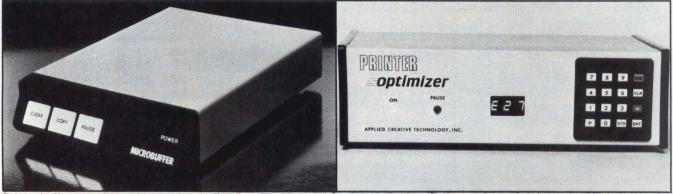
Printer buffers can do much more than buffer data. The Microbuffer (left) from Practical Peripherals Inc. controls the printing of as many as 255 copies, accepts text and graphics and permits single-sheet printing and page formatting. Applied Creative Technology Inc.'s Printer Optimizer accepts printing-control commands via its 16-key keyboard and can handle up to 99 user-programmable strings of ASCII characters and perform character translation and filtering.
