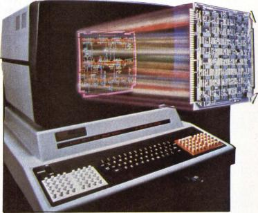
Gerber Systems Technology's CAD workstation for PC-board layout is based on the HP 1000 computer. The company plans to incorporate the HP 9000 32-bit microcomputer when it becomes available. Gerber is one of the leading suppliers of such systems.
