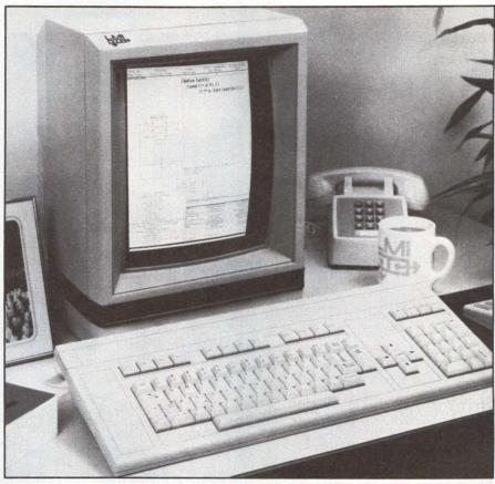
LISP Machine's Lambda LISP-based computer system is targeted at a market requiring more efficient software development using LISP programming.
