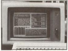
Lantech Systems Inc.'s uNETix operating system for the IBM PC and other microcomputers enables five MS-DOS application programs to run concurrently with five or more UNIX applications. Each application is displayed in a window.
