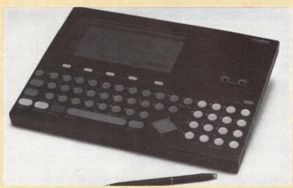
Convergent Technologies' \$895 WorkSlate notebook computer integrates an 8-bit Hitachi 6303 CMOS microprocessor, 64K bytes of ROM, 16K bytes of RAM, a microcassette recorder and a 16-line-by-46-column liquid-crystal display.
