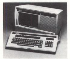
nonvolatile RAM that requires no battery backup. Data communication between the terminal and the HP host is via an RS232 interface. Data-flow control is performed with x-on/x-off or ENQ/ACK protocols. The 820's block transmissions are compatible with HP's DC1-DC2 handshake protocol. Single-unit price is \$1495, with volume discounts available to OEMs. Direct Inc., 4201 Burton Dr., Santa Clara, Calif. 95050.
