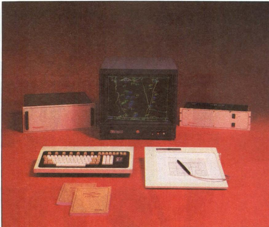
**Genisco's new 6210 high-end graphics terminal features 1392 × 1024 interlaced resolution and can display as many as 4096 colors out of a possible 16 million on a 19-in. monitor. Maximum display list memory is 1M byte.**
