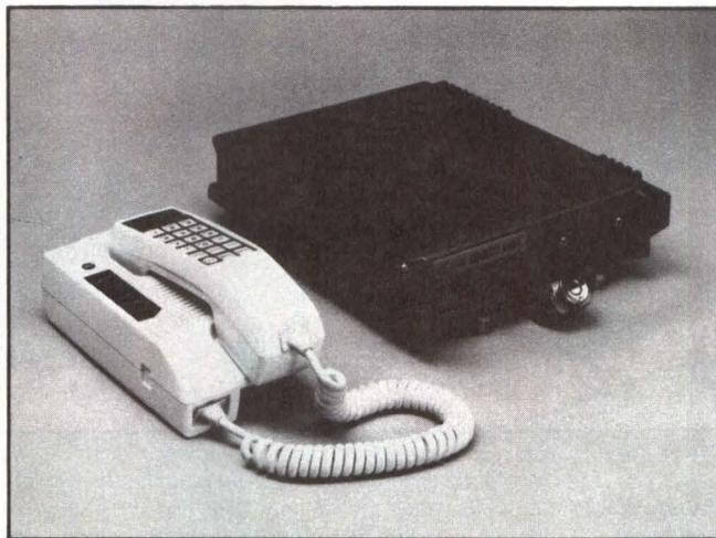
Mobile phone unit from Oki includes a handset, usually mounted within reach of a driver, and a box mounted in the trunk handling transceiver and control functions. Most mobile units are used with two antennas for optimum reception.
