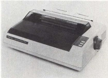
NEC Information Systems Inc.'s Pinwriter series of low-cost, dot-matrix printers features 18 printing pins to form high-density characters.
