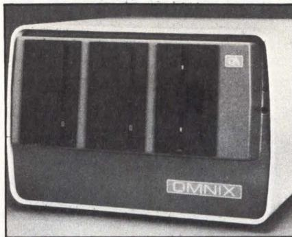
**Computer Automation's Naked Mini division** is addressing the shifting computational performance range with a 186-based system multi-user system called OMNIX 186. The basic configuration includes 384K bytes of RAM, four serial ports, a 5M-byte, 5¼-in. Winchester disk drive and a 1M-byte floppy drive for a single-unit list price of \$8990.
