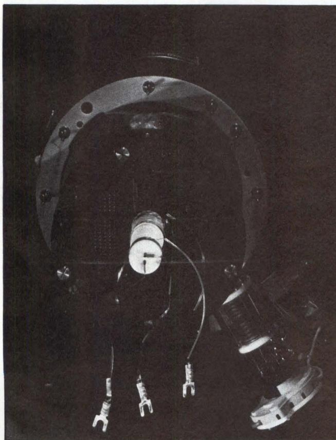
**General Electric's PJ 5055 color projector** houses a Xenon lamp, an electron gun, a light-valve chamber and a projection lens. The unit weighs only 140 lbs. and accepts RGB and NTSC color signals.
