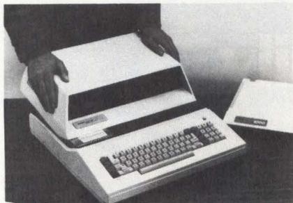
external cabling. The single-sided ACE 10 drives store as much as 143K bytes and feature an 18-msec. track-to-track access time and a 250K-bit-per-sec. transfer rate. The single-drive ACE 1100 is priced at \$699 including the controller. A second drive adds \$399. **Franklin Computer Corp.** 2138 Route 38, Cherry Hill, N.J. 08002.
