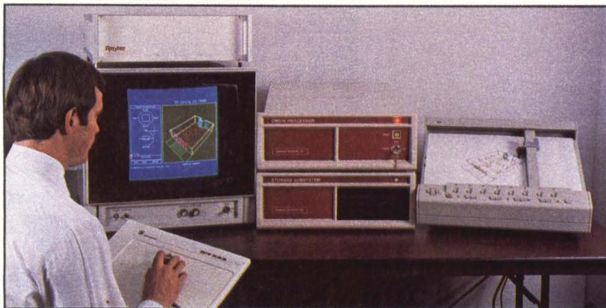
Precision Visuals Inc.'s graphics package for MC68000-based microcomputers is compatible with more than 40 output devices. The library of 160 FORTRAN routines allows such functions as 3D transformations, interactive selection of color, a pick function and segments support to be performed.
