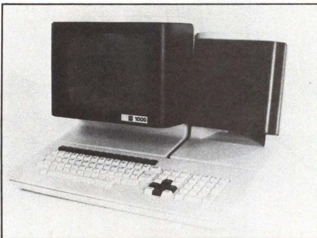
**Fig. 4. Multi-microprocessor-based small-business systems distribute processors to users or groups of users. As many as 23 Pertec 1000s (left) can be connected using Pertec's REACH local-area network. MC68000-based Tandy Corp. TRS-80 model 16s (right) can be linked using Datapoint's ARCnet and can be tied into Datapoint business systems.**
