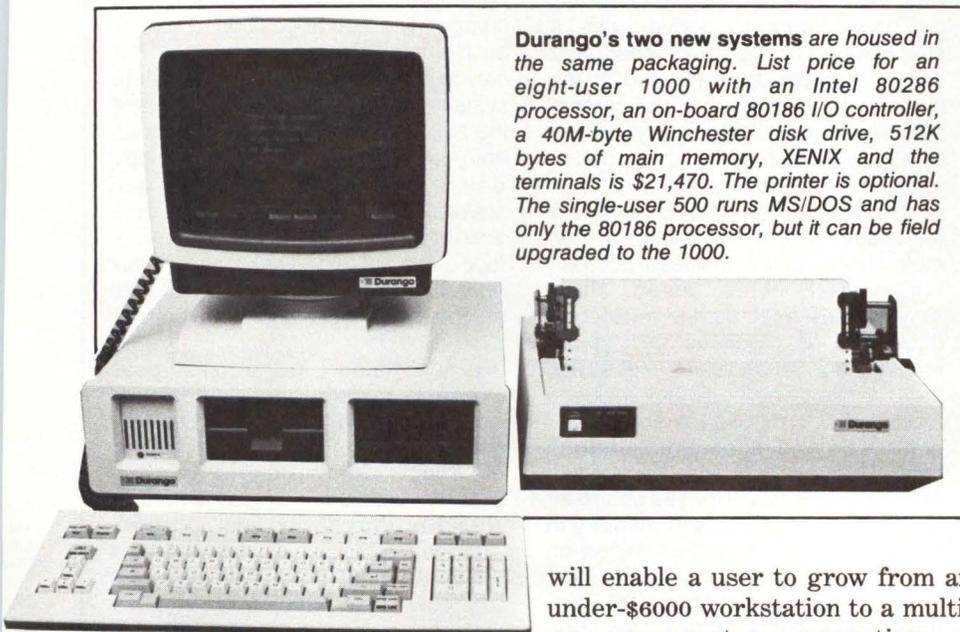
**Durango's two new systems** are housed in the same packaging. List price for an eight-user 1000 with an Intel 80286 processor, an on-board 80186 I/O controller, a 40M-byte Winchester disk drive, 512K bytes of main memory, XENIX and the terminals is \$21,470. The printer is optional. The single-user 500 runs MS/DOS and has only the 80186 processor, but it can be field upgraded to the 1000.
