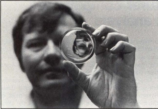
**Roger Heuppchen** examines a lens blank at Signet Optical. Because the lens molds are inspected daily to ensure proper physical parameters, the lenses need only be inspected for nine potential visual defects such as scratches and bubbles.
