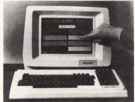
underline, bold and blink attributes. ETT terminals include a touch-sensitive screen overlay with 32 touch-sensitive areas on non-glare glass. The Touché controller supports a mix of as many as four video terminals and printers with four optional additional ports. Prices of the Touché terminal range from \$3500 to \$3900. Prices for the controller unit range from \$5650 to \$6350. **Emutec Inc.**, 908 Concord St., Framingham, Mass., 01701. **Circle No 326**
