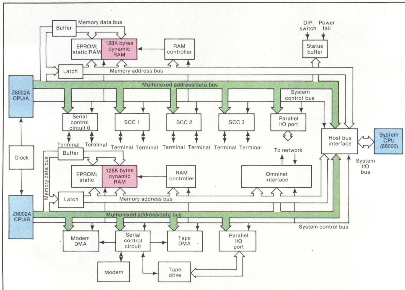
Fig. 3. The I/O interface is based on two Z8002 CPUs, one (CPU/A) controlling eight serial ports and one parallel port, and the other (CPU/B) controlling modem and network interfaces. Each CPU has 128K bytes of local RAM, which is also accessible by the system CPU.
