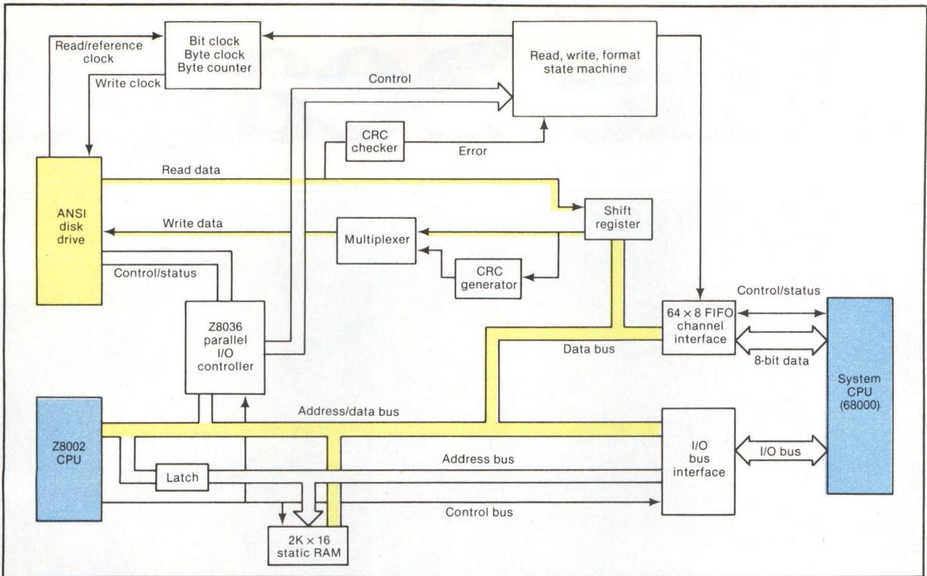
**Fig. 4. The disk interface** incorporates a Z8002 CPU that receives commands and operating software from the system CPU. Data are transferred from the disk to the FIFO channel interface buffer in bytes, and then sent to the memory in a 32-bit DMA transfer controlled by the system CPU.
