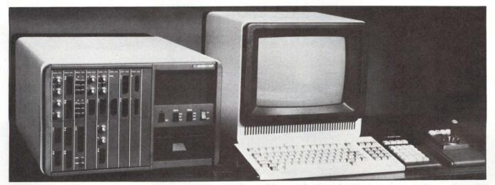
MASSCOMP MC-500 system runs an enhanced UNIX supporting real-time applications. A typical system including graphics and data-acquisition hardware and software is priced at \$40,000.
