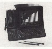
69-key standard layout keyboard with four cursor-control keys. The screen holds 24-, 40- or 80-character lines of text. The terminal also has limited graphics capability including forms and simple line or bar graphs. Housed in a cabinet measuring  $14 \times$  $9\frac{1}{2} \times 14\frac{1}{2}$  in., the Scanset XL is priced at \$895. **Tymshare**, 20705 Valley Green Dr., Cupertino, Calif. 95014. **Circle No** 331
