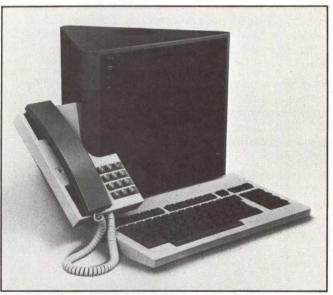
The VoiceStation 1 68008-based workstation incorporates bitmapped graphics, telephone functions and digitized voice storage for dictation. Each workstation in the Sydis system is connected to the system information manager through a 320K-bit-per-sec. dedicated line. The system is priced at \$6000 to \$7000 per user in OEM single-user quantities.
