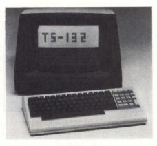
$\times$  10 characters in an 8  $\times$  12 dot-matrix cell. White and amber screen colors are optional. Special function keys, baud rates for the two ports, parity checks, conversation modes, protocols, scrolling, screen brightness, cursor type and line length are software selectable. These parameters are retained by CMOS circuitry even when the power is off. Price is \$1650 in single-unit quantities. Falco Data Products Inc., 1286 Lawrence Station Rd., Sunnyvale, Calif. 94086.
