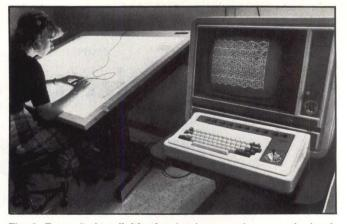
**Fig. 2. Tread-design digitization** involves entering a rough sketch through a CalComp 6482 digitizer into an Eclipse processor over a 4800-baud RS232 line. The Eclipse echoes the data serially at 9600 baud to the CRT display, and the designer modifies the tread configuration by using the keyboard to select functions and the joystick to identify segments of the image to be manipulated.
