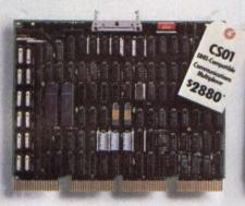
Handles 8-64 channels, 16-bit word transfers (DMA), 22-bit addressing. (16- channel price)
