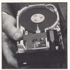
**CDC claims the thin-film-head technology** used in its 6.38M-byte 3<sup>1</sup>/<sub>2</sub>-in. Cricket Winchester disk drive is ideal for portable computers because the heads never actually touch the media, thereby lessening potential abuse.
