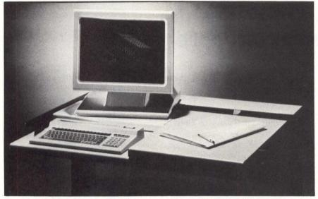
**The Sigma 6100 series of intelligent raster graphics workstations** features GKS functions built in firmware. Resolution on both the monochrome and color displays is  $1448 \times 1024$  dots. Pictured is the 6150 monochrome version.
