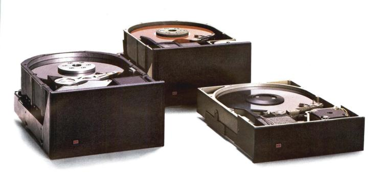
three models: 6.4MB, 12.8MB, and 19.2MB unformatted capacities. Our TM703 is a high-performance, closed-loop 51/4" drive with a full 30MB of storage.
