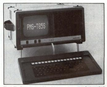
Fig. 1. The Siemens portable microcomputer system features dual minifloppy disks, a 9-in. CRT display and a detachable keyboard.
