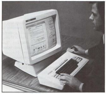
Xerox's 8010 Star professional workstation is configured with 8000 NS (Ethernet) LAN shared-resource facilities to provide integrated office-automation electronic mail/filing and communications capabilites. Datapoint's IEOS system also employs an LAN architecture (ARC) to implement and configure office-automation systems via intelligent workstations, sharing network file (disk), printer and communications resources.
