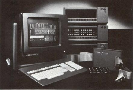
Kontron Electronics' KDS configurable development system/EE workstation features modular, ergonomic design with separate adjustable CRT and detached keyboard, computing and mass storage, universal in-circuit emulation, timing and state logic analysis, a Z80 CPU and the CP/M operating system.
