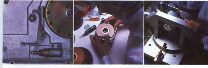
the field a snap. Spindle brake on power off, parking in datafree zone and automatic positioner latch that never requires any operator action. Making the 1300 the most reliable and easiest to service drive in the industry.
