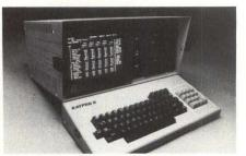
Other features include a Z80 processor, two built-in 5<sup>1</sup>/<sub>4</sub>-in. floppy disk drives that store 191K bytes each and 64K bytes of RAM. The Kaypro II uses the CP/M 2.2 operating system and includes word-processing, spelling-checker, mail-list and electronic spread-sheet application programs as well as the S-BASIC and M-BASIC programming languages. Single-unit price is \$1795. Kaypro Division, Non-Linear Systems Inc., 533 Stevens Ave., Solana Beach, Calif. 92075.
