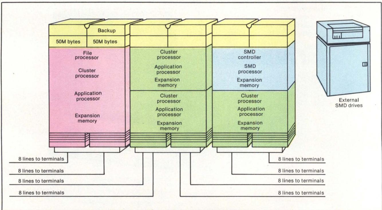
**Fig. 2. A system to serve 64 users.** A master chassis (left) and two expansion chassis, plus external mass storage, can be assembled into a system that supports 64 users. Such a system can be expanded to accommodate a maximum of 128 users, 28M bytes of ECC RAM and 1.5G bytes of integral Winchester disk storage.
