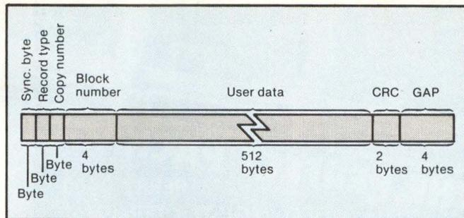
**Fig. 2. A VCR data block** combines 0.5M bytes of user data with 13 bytes of synchronization, address and error-correction information. Data blocks are recorded repeatedly in sequence for reliability through redundancy. During tape read operations, only the first error-free copy containing the expected block number is read. All subsequent copies are ignored.
