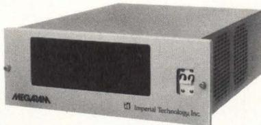
When used as a disc replacement, the high speed, non-rotating MegaRam provides the software compatibility of a disc with the performance of main memory. Ideal for swapping, scratch files, overlay storage, process control, telecommunications, graphics, data acquisition, array processing, etc.
