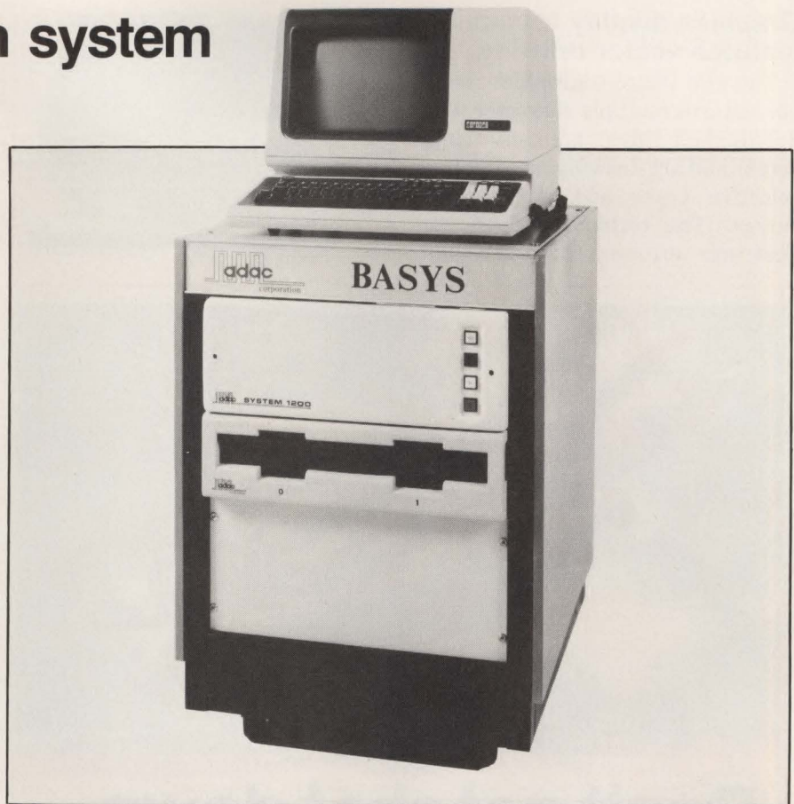
ADAC's BASYS data-acquisition and -control system is designed around a DEC LSI-11/2 or LSI-11/23 processor and is fully LSI-11 bus-compatible. The system works with ADAC's line of LSI-11, low-level and high-level analog I/O, discrete digital I/O and signal-conditioning devices.
