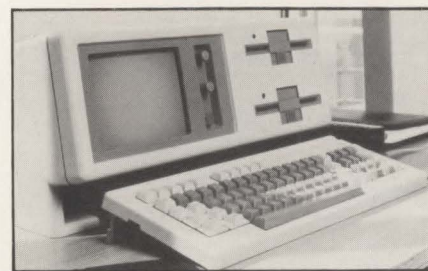
Dynalogic's Hyperion, said to run IBM Personal Computer software, is packaged in a 18- × 10- × 8½-in. package with a carrying slot for the detachable keyboard. The package was designed by Hovey/Kelley Design, which also designed the Apple III's packaging.
