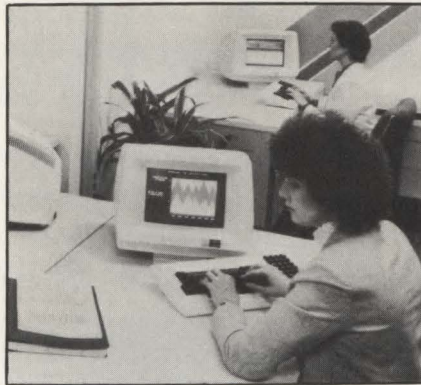
The Datamedia 932 multi-user microcomputer is based on the MC68000 and is the first such system to run the Pick operating system. Competitors will follow soon.
