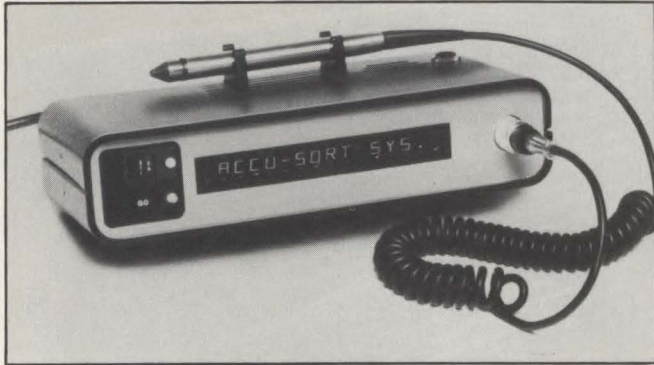
The Accu-Sort model 4510 light-pen bar-code reader sells for less than $1000 and includes a power supply, a decoder and a 16-character alphanumeric LED display. The unit is intended for factory-floor data-entry applications.
