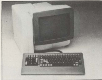
The TeleVideo 970's most striking aspect is its profile, the result of mounting the logic boards and power supply in a vented case. Vertically placed PC boards are convection cooled to give the terminal's electronics an estimated 60-percent longer life span. Another result of the design is a balanced CRT terminal that can be tilted with one finger.
