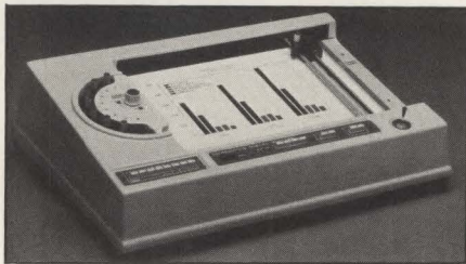
Tektronix's model 4662 option 31 eight-pen plotter offers higher output quality than plotters, and although typically slower than printers, some users will make that trade-off for quality.
