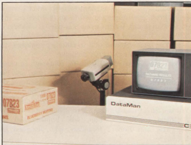
The Cognex Dataman system will be used with robots in a food-processing plant. After the Dataman reads the labels of six flavors of packaged food as the packages go down a conveyor belt, a robot directs the packages to their appropriate pallets.
