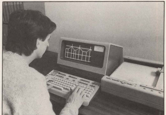
Graphics display of finite-element analysis shows deformation of mining horizon 300 ft. below surface. HP 2648A terminal and HP 1000 minicomputer have helped consultants lower computing costs and increase productivity.
