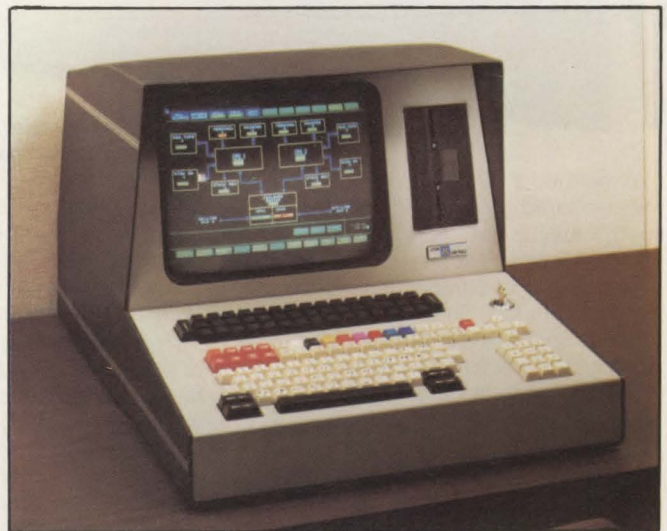
Aydin Controls is moving down into the low end of the process-control market with the 5217CT character-oriented color terminal. With an optional floppy-disk controller, the unit functions as an intelligent programmable color-graphics display or as a full stand-alone microcomputer system. Prices start at less than $5400.
