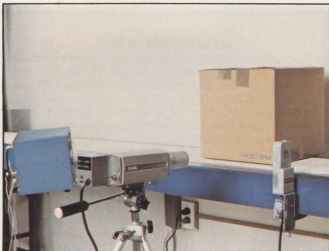
The Cognex Dataman system will be used with robots in a food-processing plant. After the Dataman reads the labels of six flavors of packaged food as the packages go down a conveyor belt, a robot directs the packages to their appropriate pallets.
