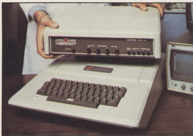
ISAAC system allows Apple II to be used as a personal laboratory work station, performing a variety of data-acquisition-and-control tasks. It is available as an Apple add-on or complete with 48K-byte Apple and peripherals.
