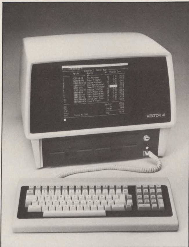
Vector Graphic Vector 4 microcomputer uses 8-bit Z80 and 16-bit 8088 microprocessors to support CP/M 80 and four 16-bit operating systems. Dual floppy drives or a floppy and a 5M-byte Winchester are mounted in base.
