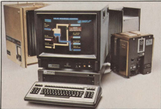
The ruggedized Industrial Data Terminals Corp. 2200 series display includes bubble memory with as much as 256K bytes of nonvolatile memory. Prices for the display start at $11,500.
