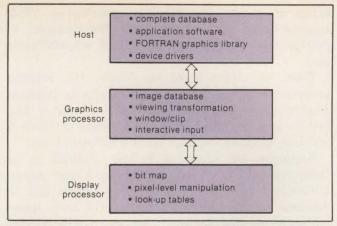
Fig. 3. Distribution of 8100/GS software functions leaves the host processor free of image-drawing and manipulation functions and of input interrupt processing, all controlled by graphics-processor software. Display-processor software converts graphics-processor commands and image-segment attributes into pixel-level data.
