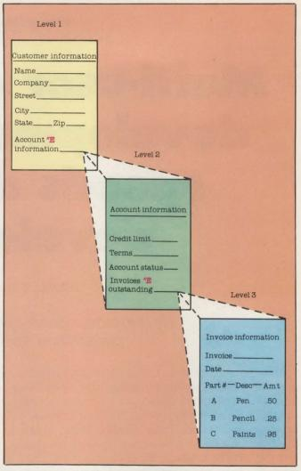
Fig. 4. Form-within-a-form mechanism allows a user to expand one field into an entirely new form. Any and all fields designated as a form within a form can be expanded into a separate form by hitting "Control E." The new form can occupy an entire screen, or a split screen along with the form that called it. Every form expanded from a single field can have any or all of its fields expanded into other forms. The process can be implemented five levels deep.
