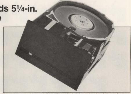
Latest additions to Seagate's ST-400 line of 5¼-in. Winchesters include the single-platter, 6M-byte ST-406 and the 19M-byte, three-platter ST-419. The 12M-byte, two-platter ST-412 (above) was announced this year in the wake of Seagate's decision to drop the ST-512, the first small Winchester to use thin-film read/write heads. All ST-400 series drives use shorter gap length manganese-zinc ferrite heads.
