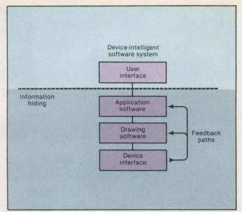
Device-intelligent software has the same four modules as device-independent software, but feedback paths provide application and drawing software with information on output-device characteristics from device-interface software. Images can be optimized for one device and previewed on another. Information hiding occurs only between user interface and other modules, keeping process user-transparent.
