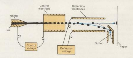
Fig. A. Continuous-jet system.
