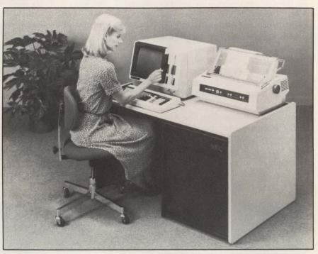
NEC Information Systems Advanced Personal Computer is based on Intel Corp.'s 8086 16-bit microprocessor. In a basic 128K-byte version with a monochromatic screen and a 1M-byte, 8-in. NEC floppy-disk drive, it carries a list price of \$3298.
