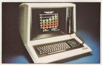
Fig. 1. The Ramtek 6211 intelligent graphics terminal features integral microprocessor and memory, a detachable keyboard and a light pen. The terminal displays 16 simultaneous colors from a palette of 64 and sells for about \$6000.
