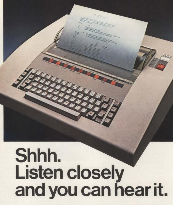
It's a pleasant sound. No clicking or clacking. Little more than a gentle rustle that's usually masked by other ambient noises. The IBM 3232 Model 51 has a non-impact, multi-element matrix print head. Instead of banging away at the paper, imaging is done by electronically removing dots from the special aluminum-coated paper, exposing easy-to-read characters.
