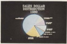
Pie chart created with IGS is constructed with simple commands. Slices can be filled with a variety of patterns in different colors.
