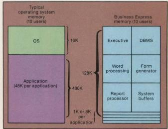
Fig. 2. Memory requirements for individual Business Express users are 2K for database applications and 8K for word-processing applications. All modules required to process applications reside in RAM, requiring user memory only for current program data. For a 10-user system, a traditional operating system typically requires a minimum 496K of memory compared to 196K for Business Express.
