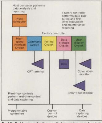
Gould's first-level production monitoring system uses four independent processor modules called Cybloks.
