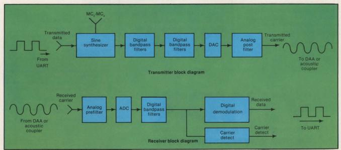
Advanced Micro Devices' Am7910 modem chip uses digital signal processing techniques to perform modulation, demodulation and filtering functions. On-chip analog-to-digital converters (ADC) and digital-to-analog converters (DAC) in conjunction with a digital signal processor eliminate the need for external analog filters. (UART = universal asynchronous receiver/transmitter; DAA = data access arrangement)
