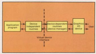
Fig. 1. Device-independent graphics software modules keep applications programs from becoming obsolete as hardware environments change. Application programs call on standardized, device-independent graphics routines. Dedicated device managers for each I/O device translate these device-independent commands into device-dependent commands. To take advantage of a new or better I/O device, a user need only write a device manager for it. His application program does not change.
