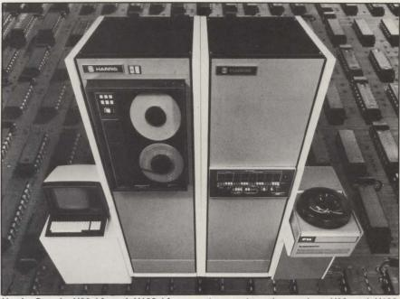
Harris Corp.'s H80-1A and H100-1A computers replace the previous H80 and H100 computers and feature the new VOS operating system, 768K bytes of executable address space and high-density memory.
