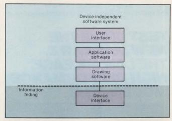
**Device-independent software** consists of four modules. Information in device interface software is hidden from other software, so that displays are created independently of output device characteristics.
