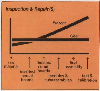
As part of its effort to reduce manufacturing costs, Tektronix will carry out inspection activities throughout the assembly process. In doing so, the company hopes to reduce the cost of repairing a finished product.
