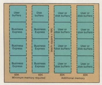
Fig. 3. Memory is allocated in 16K increments to user buffers or disk buffers. Allocating memory to user buffers allows as many as 20 users to operate the system concurrently. Allocating memory to disk buffers keeps the performance of the system high. The best rule of thumb is to use the smallest number of 16K blocks that supports the number of users operating the word processor concurrently, at two word-processor users per 16K, and allocate the rest of the 16K blocks to disk buffers.
