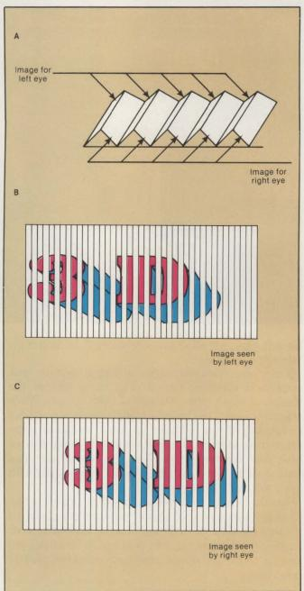
Lenticular images, used for hard-copy production of 3D images, use a surface divided into thin, multi-sided ridges (A). One image is displayed on the same side of each ridge, and another image is displayed on another side. Several images can be displayed on one surface (a two-imaged surface is depicted here). When viewed at the appropriate angle and distance, each eye sees a different set of ridge sides, and thus a different image, for a true 3D effect.
