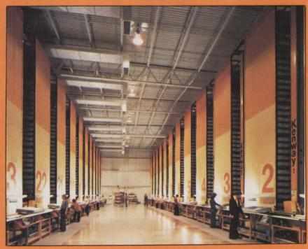
Approximately 65 percent of the 130,000-part lines stored in the automated Tektronix warehouse are housed in the miniload section. Two DEC PDP 11/70 computers keep track of where each part is in the storage process.
