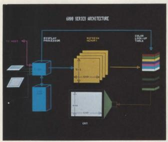
Fig. 2. 6000 series architecture. Graphics input from a host computer or from the terminal's keyboard, graphics tablet or light pen is processed by a Z80 microprocessor. The processed data draw graphics into the screen's refresh memory, program the video look-up table, or are stored for later recall. Graphics drawn in the refresh memory are assigned colors via the look-up table, and are converted to analog signals that are displayed on the CRT screen.
