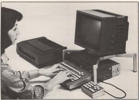
Sony's SMC-70 personal computer is based on the 8-bit Z80A microprocessor, but is available with an 8086 upgrade card for about \$1000. The basic version is priced as low as \$1475 with 64K bytes of program/data RAM, 38K bytes of graphics memory and a separate 32K-byte system memory.
