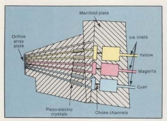
Fig. 1. The ACT-1 ink-jet print head is a modified version of the Siemens PT80i. Shown here in section, the head is divided into three sets of four jets. Using inks in the three subtractive colors in combination, the additive primaries (red, blue, green), as well as black, can be produced.
