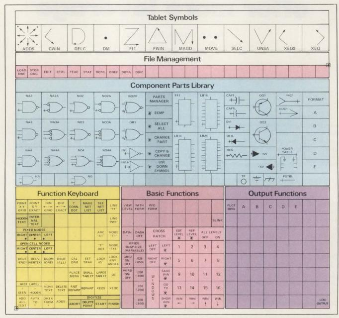
Schematic-drawing tablet overlay allows Applicon users to draw, move, delete and align symbols with only a few touches of a stylus. Other tablet areas are used for file management, system commands, output management and other user-defined command sequences.
