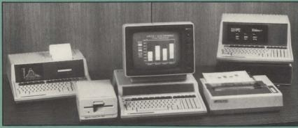
**Hewlett-Packard Co.'s Series 80 family of personal computers** now includes (from left) the portable HP85, the HP86 and the HP87XM, with 128K bytes of built-in user memory.
