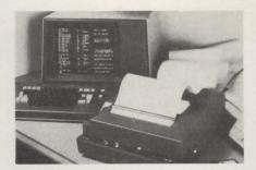
alphanumeric and graphics capabilities. The unit prints 80-character lines at 240 lpm or 320 cps and produces a 24-line CRT screen page in less than 6 sec. Price is \$840 in single-unit quantities and \$470 in quantities of 500. Olivetti OPE, 505 White Plains Rd., Tarrytown, N.Y. 10591. Circle No 348
