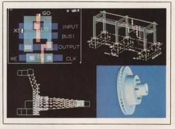
Applicon packaged software is available for general-purpose and specialized applications. Clockwise from top left are screen output from a circuit-layout package, a drawing-dimensioning package, a solids-modeling package and a stress-analysis package. Because they can amortize software-development costs over large user bases, turnkey vendors can sell most packages for far less than users could pay to develop them in-house.
