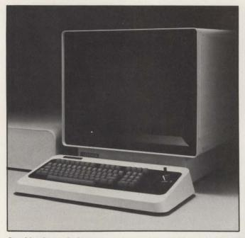
**Graphics input devices** are an important part of ergonomically designed work stations. The CalComp IGS workstation (right) uses a joystick, a tablet, and a keyboard. The Lexidata 2400 (above) uses a keyboard supplemented by an integral joystick.
