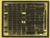
• 4 MHz Z-80A CPU • Two banks of 64K RAM • Two RS-232 serial ports • Full centronics printer port • True hard disk interface • External DMA I/O • Compatible with 5 inch and 8 inch drives, single/double density • Real time clock• 5 volts only at 1.5 amps • Com-pact size • Source Listings are included
