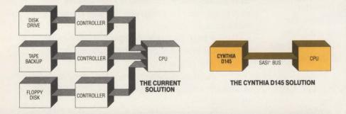
Utilizing the processing power of the intelligent, SASI-compatible interface, the Cynthia D145 20MB (24MB unformatted) drive handles all error handling and protocol interface functions... without separate hardware interfacing or applications software changes. It's all handled by the drive, at the system level, totally
