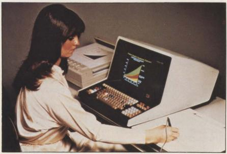
The 8000l graphics system supports IGS software for I/O device-independent graphics. Available peripherals include plotter, digitizer and color ink-jet printer.
