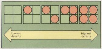
Fig. 2. Dithering is a technique used to reproduce different intensity levels of the same color. Each pixel on a graphic system's monitor is represented by four dots on the hard copy arranged in a  $2 \times 2$  dot matrix, as above. By varying the number of dots printed from zero to four, five levels of color intensity can be produced for each of the three primary colors. When combined, these generate 125 color shades.
