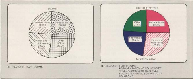
Fig. 1. Standard pie chart drawn with SPSS graphics. A user can request a standard chart that uses default parameter values (a) or can enter commands to customize the chart (b).
