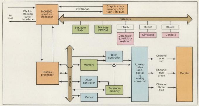
Fig. 2. Lexidata 8100/GS graphics processor consists of a 16-bit graphics processor with graphics and database manipulation capabilities and a display processor for converting vector commands to raster data. Input device interrupts are also processed by the graphics processor, leaving the host free for applications software and heavy computation.
