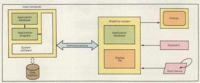
Fig. 1. Distributed-processing graphics system structure consists of a host and a separate processor for graphics manipulations. Graphics database information can be down-loaded from the host to the graphics processor, so that user modifications to the image are processed locally. Input devices can also be supported locally, and data are transmitted to the host through large buffers.
