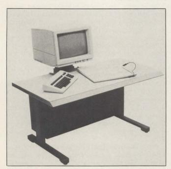
Fig. 2. Applicon's Series 4000 work station stresses simplicity and ergonomics. The multi-plane display generates graphics and alphanumerics. The tablet and stylus can be used for graphic input or command menu selection. The 19-in. display module tilts, swivels and adjusts vertically on a pneumatic column. The work surface measures  $30 \times 60$  in., is low glare and is height-adjustable.
