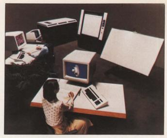
Fig. 1. Applicon's Series 4000 turnkey CAD/CAM system is built around a Digital Equipment Corp. PDP-11 or VAX minicomputer and Applicon's proprietary graphics processor. Single-workstation, black-and-white systems sell for less than \$100,000. Applicon offers more than 120 general-purpose and application-specific software packages from the Series 4000, which also runs third-party software.
