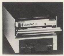
word processors and business and general-purpose minicomputers provides 16M bytes of removable storage and 32M bytes of fixed storage. The drive features one removable disk and three fixed disks, a data-transfer rate of 1.208M bytes per sec. and an average seek
