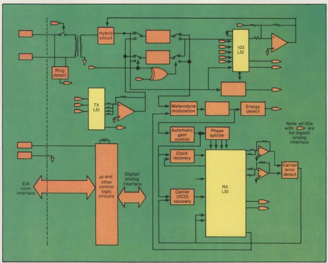
This block diagram of a modem under development at Racal-Vadic illustrates how modem manufacturers are increasingly relying upon various LSI components in their product designs. The 103 LSI chip is the TMS99532 jointly developed by Racal-Vadic and Texas Instruments, and the transmit (TX) and receive (RX) components are custom chips jointly developed by Racal-Vadic and RCA. The microprocessor is an 8-bit Intel 8048.
