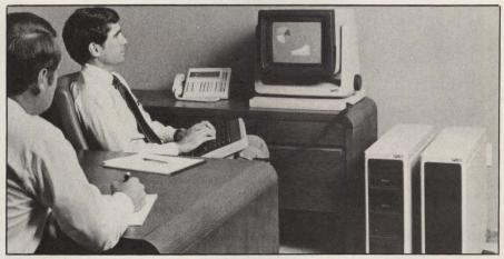
One of the newest entrants in the mid-range graphics terminal market is the Florida Computer Graphics Beacon. The product is built modularly for expansion and integrates data-processing, word-processing and data-communications functions with graphics.
