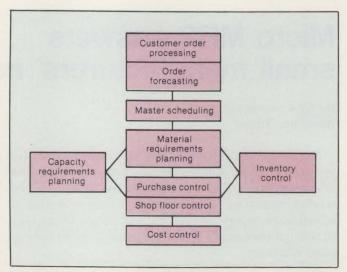
The major functions of a commercial system show the system's typical image. Source: Computer Aided Manufacturing-International, Inc.
