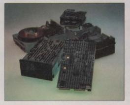
Features: Buffered/slew seek modes - Automatic seek and verify □ Automatic head and cylinder switching = 256/512 bytes per sector ☐ Multiple sector buffering ☐ Odd parity checking D Logical sector addressing and interleaving ☐ Autonomous error detection and correction with retries □ Automatic tape read retry on error
