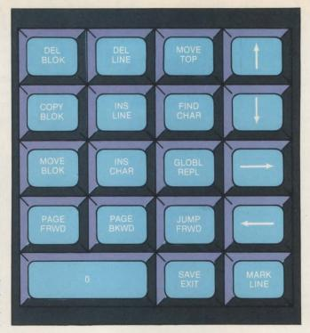
Function keys are used to execute popular commands in most word-processing packages. The keypad above is from a Digital Equipment Corp. VT-100-compatible terminal running Unique Automation Products' EZEDIT/WP, a full-screen text editor used with the company's EZTYPE text formatter to perform word-processing on DEC LSI-11 and PDP-11 minicomputers.
