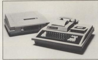
Fig. 4. Self-sufficient portable teleprinters are a kind of intelligent terminal. This International Entry Systems, Inc., Datacorder I packages a modem/coupler, minicassette recorder, 16-character display, 80-column 5 × 7 electrostatic printer and a Z80 μp with 16K to 32K bytes of RAM in a 5½- × 17½ × 18½-in. briefcase. Computer Devices and others offer similarly powerful units.
