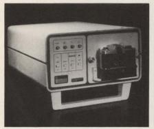
The device features digital RGB color input resolution and a rearpanel, 10-position, push-button switch that adjusts film speed and color characteristics. Single-unit price is \$4490, with OEM discounts available. Image Resource Corp., 2260 Townsgate Rd., Westlake Village, Calif. 91361.
