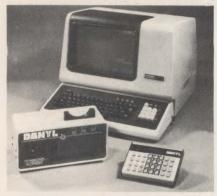
via keypad or badge, one or more ID codes that open the CRT and allow it to transmit. User ID, applicable accounting codes and transaction time are recorded on a cassette tape. The device connects via RS232 ports. Danyl Corp., Pennsauken, N.J.. Circle No 331
