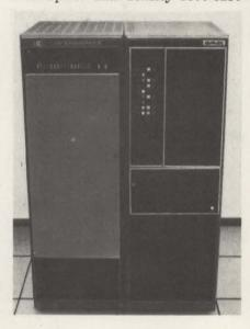
bpi tape subsystem supports H-P's series 64, 44, 40, 30 and 33 computers. The streaming capability incorporates two 16K buffers that enable continuous disk-to-tape data transfer and enables the tape system to do a 100M-byte write in approximately 3 min. The system provides 125-ips tape speed and 590K-byte burst rate. Price is \$45,500. Qualex Technology Inc., 31220 La Baya Dr., Suite 110, Westlake Village, Calif. 91362.
