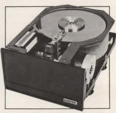
Evotek's line of high-capacity, high-performance 51/4-in. Winchesters range in capacities from 7.8M to 51.6M bytes. The drives operate at access times of 65 msec. using a stepper-motor actuator. Drives using voice-coil motors may be expected later on from the Fremont, Calif., start-up.
