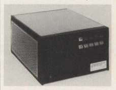
memory, 12.5M bytes of Winchester-disk storage, 0.6M bytes of floppy-disk storage, four serial channels, a video terminal and the RT-11 operating system. Singlequantity prices are \$350 for the
