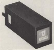
The devices need no filament adjustments and feature modular assembly. Message brightness is 100 foot Lamberts. Price is less than \$1 per message in quantities of 10,000. Industrial Electronic Engineers, Inc., 7740 Lemona Ave., Van Nuvs. Calif. 91405.
