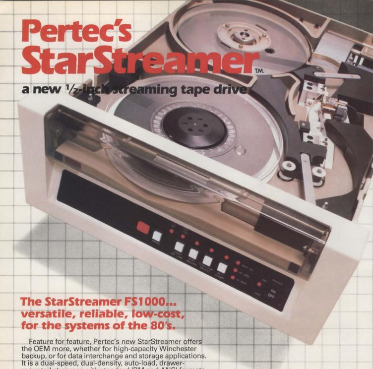
mounted streamer with standard IBM and ANSI formats. It accommodates existing software when operated at 25 ips, or operates as a high-speed streamer with transfer rates to 160 K-Bytes/Sec.
