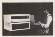
System 83 versions range from floppy-disk based systems at \$8295 to the multi-user/multitasking System 83/40 with a DMA controller and 40M bytes of memory on a Winchester disk. The System 83/40 has hardware and software to support eight ports and is priced at \$23,950. Dual Systems Control Corp., 720 Channing Way, Berkeley, Calif. 94710.
