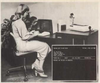
Fig. 4. Message is entered via a keyboard at a video terminal that provides a standard form (inset) for the purpose.
