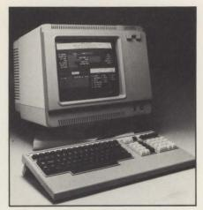
First in-house peripheral from Tandem Computers, Inc., Cupertino, Calif., is designed to meet what company executives feel will be soon-to-come rules and regulations governing safety and comfort of operators of computer terminals. Called the 6530, it incorporates a tilting, pivoting monitor and a two-position elevated keyboard with palm rest among other ergonomic features.
