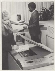
Complete black-and-white publications can be "published" in hours with Xerox's graphics system. The 1050 graphic-input station (foreground) electronically scans, digitizes and transmits images to an 8700 or 9700 laser printer (background), where graphics are merged with text and printed at speeds as fast at 120 pages per min. The 8700 also can be linked to data processing computers for high-quality printing at up to 90,000 dots per sq. in. resolution.
