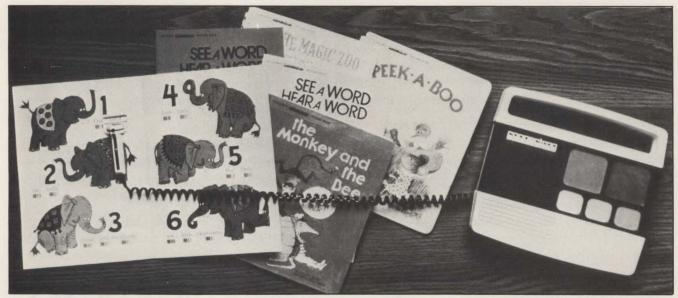
Fig. 9. "What's this word, Mama?" is a question handled by Connectron, an electronic learning aid used in Western Publishing's "New Dimensions in Learning" program. When Connectron's wand is used to scan the bar code printed under each word, the word is spoken in a friendly voice.
