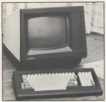
modes and protect-mode operation are standard. The system displays five hidden attributes-dim, underline, blink, inverse video and blank (security fields)-and smoothscrolls up and down, at six or 12 lines per sec. It also has a screen-saver feature that automatically decreases display brightness to zero after 10 min. of terminal inactivity. Upon receipt or entry of any data, the screen's brightness returns to normal without losing displayed information.
