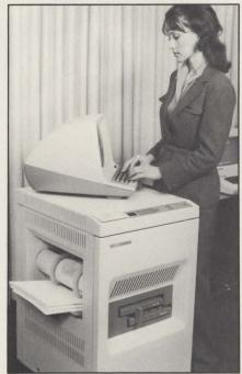
The operator is starting communications between the 2700 distributed laser printer and a central computer. The small 2700, with prices beginning at \$18,995, also can be used for output with small business or minicomputer systems.
