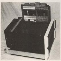
interface card. The system sustains a maximum transfer rate of 834K bps from two simultaneous HSD II cards. The memory is available in a 7- or 153/4-in, vertical chassis. The 7-in, chassis accommodates 0.5M to 8M bytes, and the 153/4-in. chassis accommodates as much as 32M bytes of error-correcting NMOS memory. Two chassis can be daisy-chained to accommodate as much as 64M bytes. Battery backup is optional. Applied Data Sciences, Inc., P.O. Box 344209, Dallas, Texas 75234. Circle No 334
