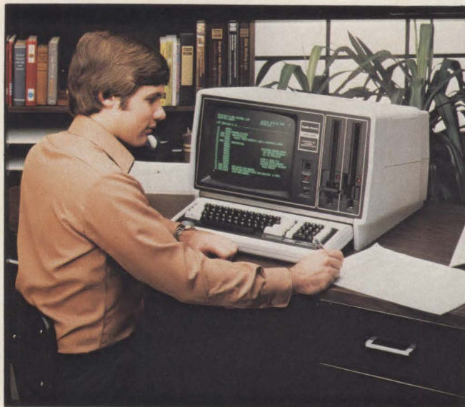
The Radio Shack TRS-80 model 16 can run 8- or 16-bit software, yet its multiterminal capability seems like a minicomputer feature.
