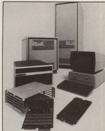
H-P's A600 \mu c and A700 mini are software compatible with the company's current 1000 products. Both use new processors based on four bit-slice devices.
