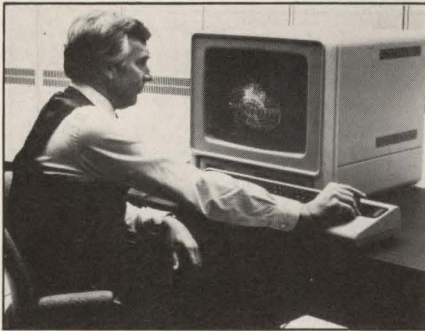
Digital Equipment Corp.'s VAX-11/782, which consists of dual VAX-11/780 32-bit processors and 2M bytes of MA780 shared memory, is designed for multistream, computation-intensive applications. One application is structural/mechanical design using a VS11 interactive color-graphics terminal.
