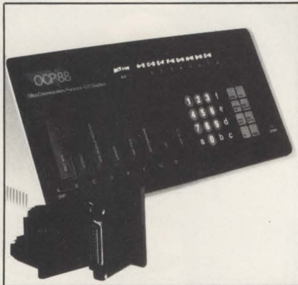
A single-line LED display on the OCP/88 indicates which systems are connected and in which direction data are flowing.
