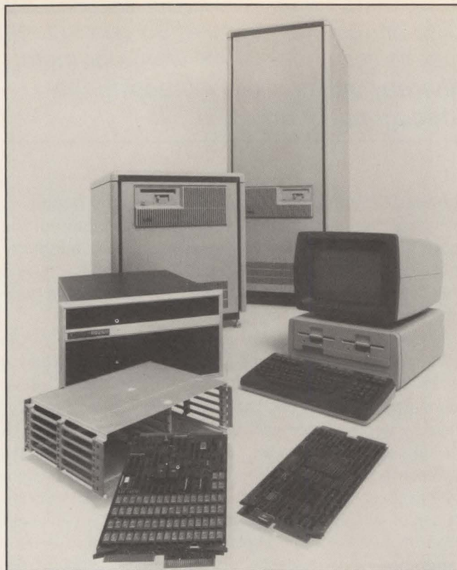
Fig. 2. Hewlett-Packard Co.'s new OEM A600 \mu c and A700 minicomputer are available in board, box and system configurations.
