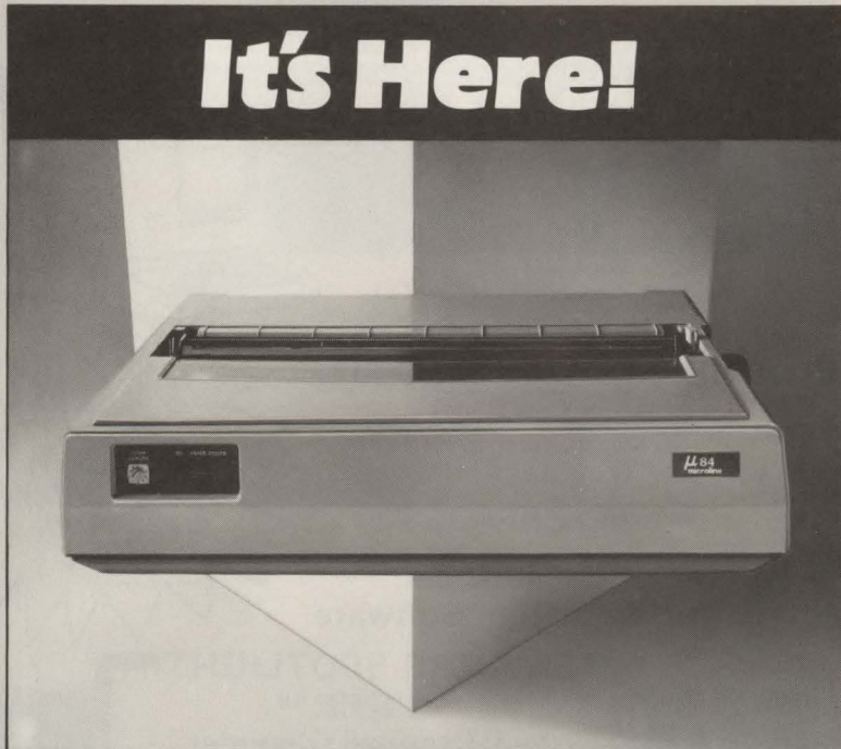
ML-84: Now available in production quantities, the multi-functional 84 offers correspondence quality and data processing throughput! 200 cps bidirectional printing, six program-selectable character sizes with true descenders, enhanced and emphasized print, proportional spacing, Okigraph™ dot addressable graphics. 9x9 matrix in draft mode, 13x17 matrix in high resolution mode. This one does it all.
