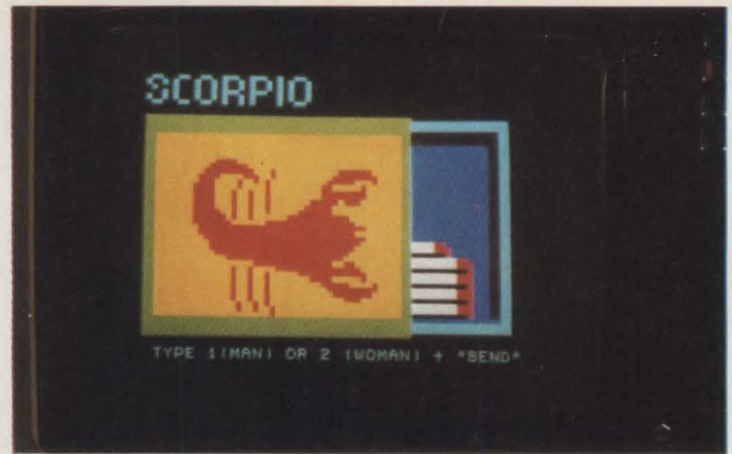
Alpha-mosaic graphics generation , as in this sample from Videodial, Inc., appears stair-stepped and not as smooth as the other major videotex method, alpha-geometrics.
