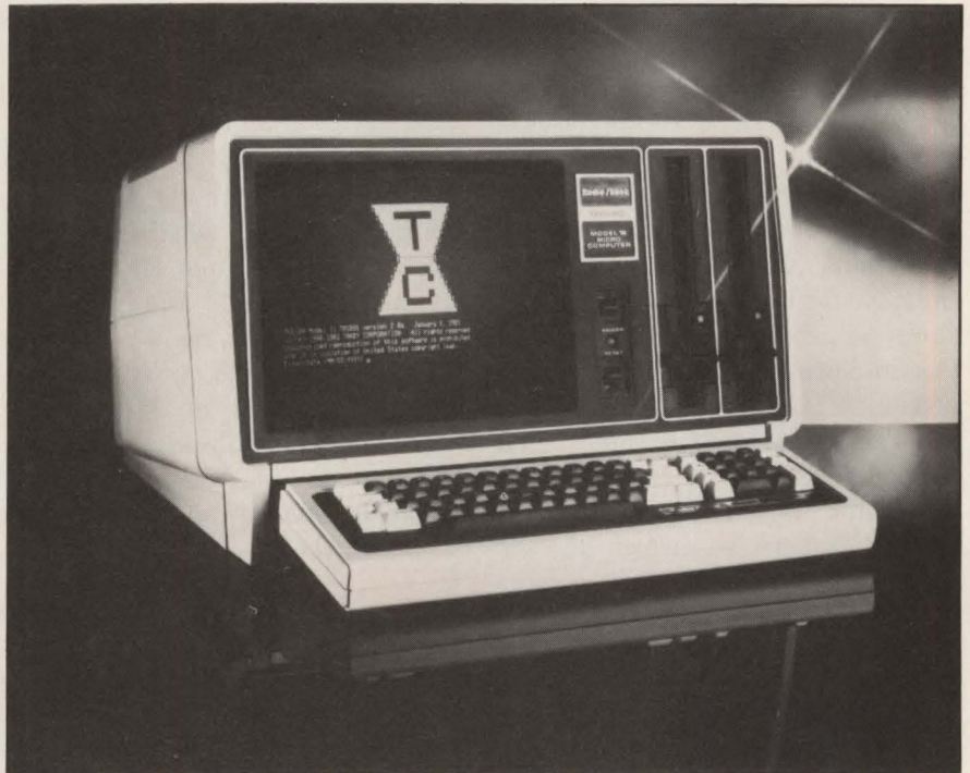
Tandy's first 16-bit \mu c , based on a Motorola MC68000 \mu p, can include as many as three terminals, and can be expanded for a total of 512K bytes of memory.
