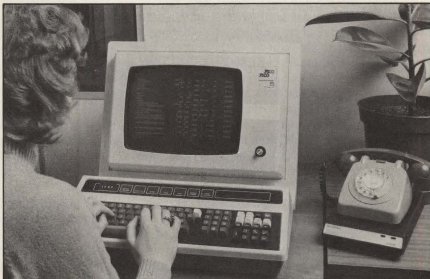
Planet local-area network from Racal-Milgo includes the terminal access point (under telephone), which can link one or two RS232 devices to the other devices on the ring network.
