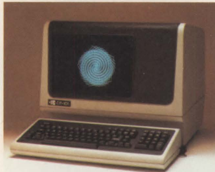
The CIT-101, which emulates Digital Equipment Corp.'s VT-100 display terminal, adds graphics capability via a plug-in graphics board. The terminal is priced at $1995; the color board is $1595.
