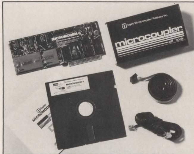
Fig. 3. Board-level modems are available for many medium- and high-volume applications. Rockwell International's R24DC (direct connect) is an FCC-registered, 2400-bps modem (l.) intended to be integrated into \mu p-based equipment. The R24DC measures 5 x 7.85 in. and is priced at $450 in small quantities. The Micromodem II (r.) from Hayes Microcomputer Products, Inc., is a 110- or 300-bps, FCC-approved, Bell 103-compatible modem that plugs into an Apple II \mu c chassis. Also included in the Micromodem II's price is the Microcoupler, a device that substitutes an RJ11C connector for an acoustic coupler.
