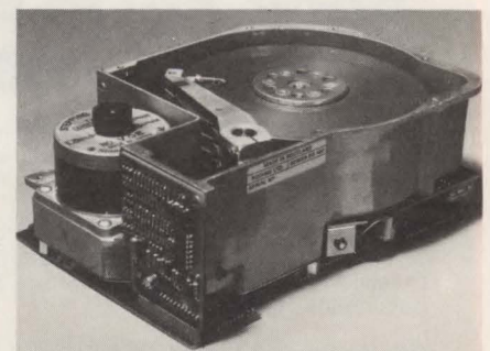
Ampex's Pyxis is available in four capacities, ranging from 4M to 16M bytes.
