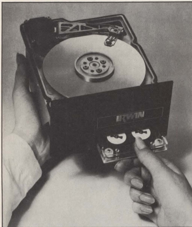
Integral 5 1/4-in. Winchester backup is the distinguishing feature of Irwin International's 510. The unit can back up its 12.3M-byte capacity on one cartridge tape in less than 4 min. The unit weighs only 5 lbs. and occupies the same space as one 5 1/4-in. floppy-disk.
