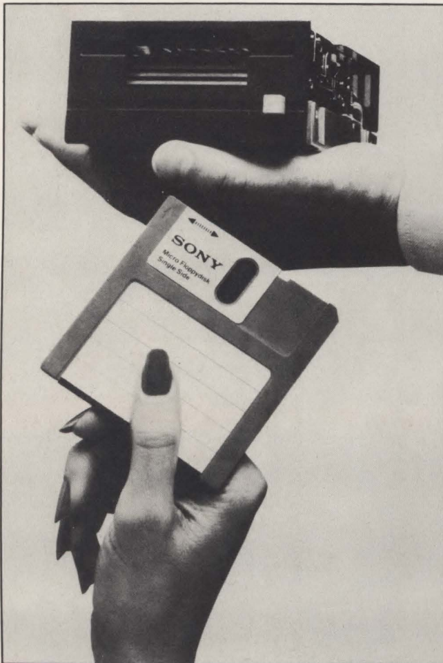
Fig. 3. Sony's 3½-in. Micro Floppy disk stores 437.5K bytes per disk and measures 2 × 4 × 5.1 in. For word-processing, personal and business applications, the drive uses a video-type precision head.
