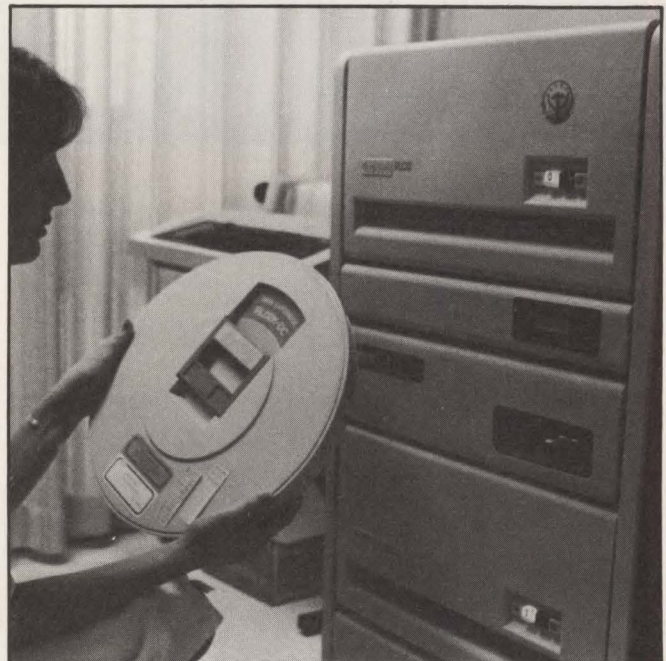
Automated psychological testing system incorporates Digital Equipment Corp. LSI-11/23 \mu c with 256K bytes of main memory and two 10M-byte RL02 disk drives. Garcia loads disk with interactive psychological testing programs.
