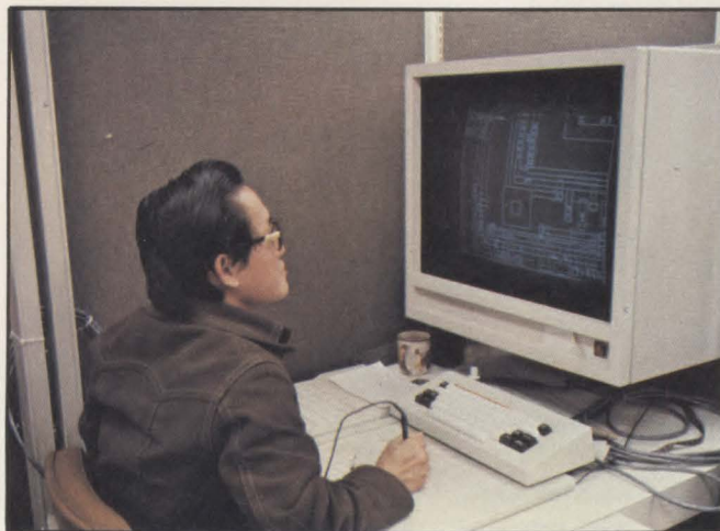
Designer Cahil Un Tak uses applications graphics terminal to lay out section of VLSI circuit. He locates circuit elements, then transfers section to a DEC VAX-11/780 supermini for design-rule and continuity checking.
