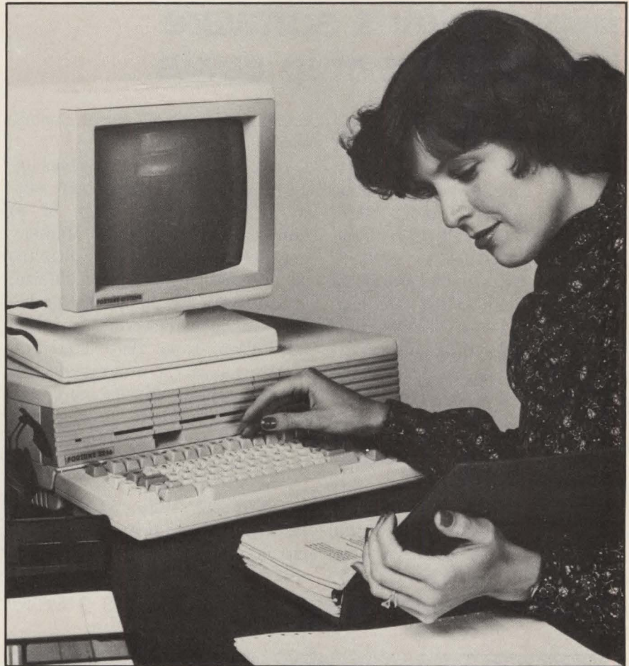
The 32:16 Motorola 68000-based desk-top computer runs Fortune's adaptation of Bell Laboratories' UNIX operating system and sells for $4995.
