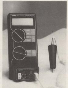
devices with a 15-mm. LCD. The unit includes an adapter for subminiature thermocouple connectors and a thermocouple sensor with a bananaplug, jack-type input. Other features include an analog output, a built-in ice point, temperature range of -40°F to 1999°F and -40°C to 1370°C, 0.1° resolution to as much as 200° and sensor interchangeability. Omega Engineering, Inc., Omega Group Co., P.O. Box 4047, One Omega Dr., Stamford, Conn. 06907.
