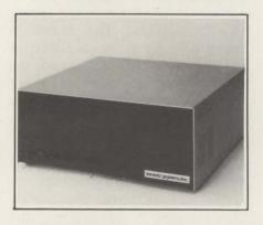
supply and the LSI 500 series controller. An off-board host adapter enables the unit to be connected to almost any CPU or bus. As many as three additional Winchester-disk drives can be added to the system, with no software modifications. Price is \$3750. Laredo Systems, Inc., 669 Giraudo Dr., San Jose, Calif. 95111.
