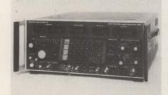
assembly. The unit features a cavity-tuned oscillator that provides sideband noise at more than -136 dBc per Hz at 20-KHz offset in the 256- to 512-MHz range, +19-dBm output level across the full frequen-
