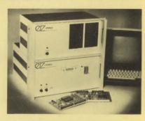
The EZ-PRO Development System supports In-Circuit emulation of over 30 microprocessors at full rated clock speed and without wait states. Processors supported include the 6800, 6802/8, 146805E2, 6809, 68000, Z80, Z8001/2, 6502/12, 6503-15, 3870/2/4/6, 8X300, 8080, 8048 family, 8085 and 2650. All bit slice devices are also supported. Prices start at \$8500 for a complete system including one In-Circuit Emulator and all required software. CIRCLE NO. 206 ON INQUIRY CARD
