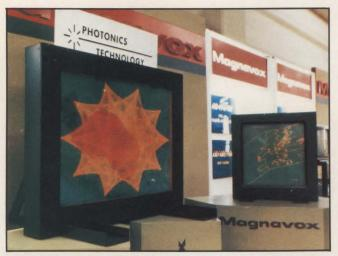
Although flat-panel displays are typically compact, Photonics is manufacturing large-screen AC plasma units for military applications. Assembled by Magnovox, the largest terminal (I.) measures 1m. diagonally and contains 2 million light-emitting pixels. The other one measures 17 × 17 in. and contains 1 million pixels.
