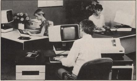
The DRS 20-series model 50 file-processing system from ICL, Inc., with an optional work-station desk (foreground), provides fixed-disk storage capacities of 16M or 27M bytes.
