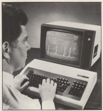
Intelligent keyboard: New graphics terminal package from Digital Equipment Corp. specifically designed for the education market provides economical interactive graphics. Called GIGI (General Imaging Generator and Interpreter), the unit is packaged in a keyboard that can be used with a user-supplied video monitor to make a terminal for use with DEC's PDP-11, VAX-11 and DECsystem-20 computers. GIGI has both color and black-and-white capabilities, depending on the monitor used.
