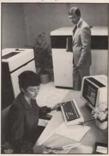
Stratus Computer's continuous-processing system is based on multiprocessors, so that each processor module is redundant.
