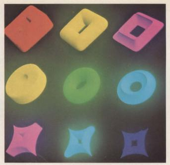
Examples of full-color imaging using 24-bit-per-pixel resolution. These "super-quadric" solids are building blocks for complicated sold shapes used in mechanical CAD.
