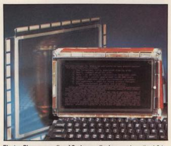
Electro-Plasma supplies AC plasma displays such as the 1.9-in-deep RS 256/512-1 (above). The display, which includes the glass and display electronics, has a 4.1-  $\times$  8.25-in. active area and handles both graphics and alphanumerics with a resolution of 62 pixels per in. Prices start at \$3450.
