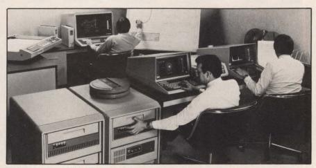
**Tektronix, Inc.'s 4909 file-management system** allows shared access to large-capacity mass storage by as many as 10 4050 series desk-top computers and features public and private work spaces, indexed files, concatenated volumens and variable-length volumes.
