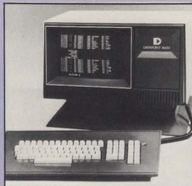
Displaying 24 lines \times 80 columns, the 8600 processor permits 16 levels of screen brightness. The keyboard can be placed as far as 1m. from the terminal.
