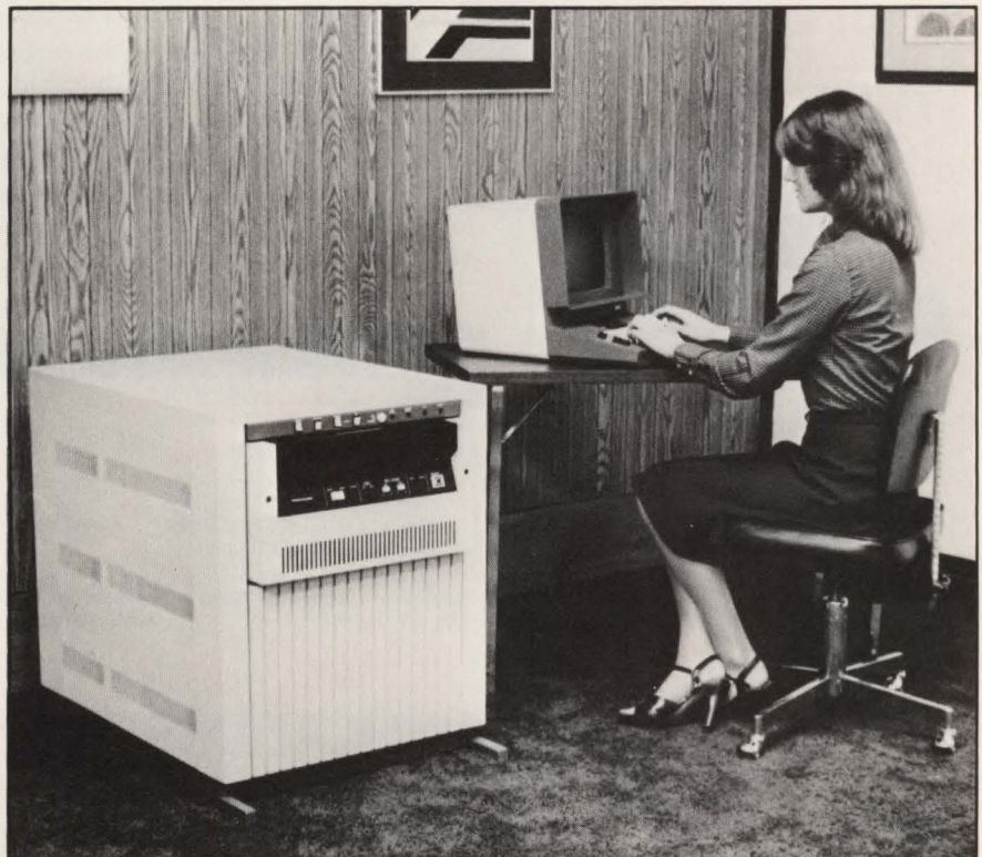
The basic 3210 system , designed for commercial use, includes a CPU, 512K bytes of memory, 16M bytes of cartridge-disk storage, 16M bytes of Winchester-disk storage and a console terminal.
