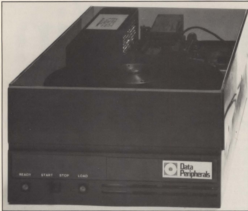
Data Peripherals has entered the fixed-medium 8-in. Winchester-disk-drive market with the 40M-byte DP400, nicknamed the Puma.
