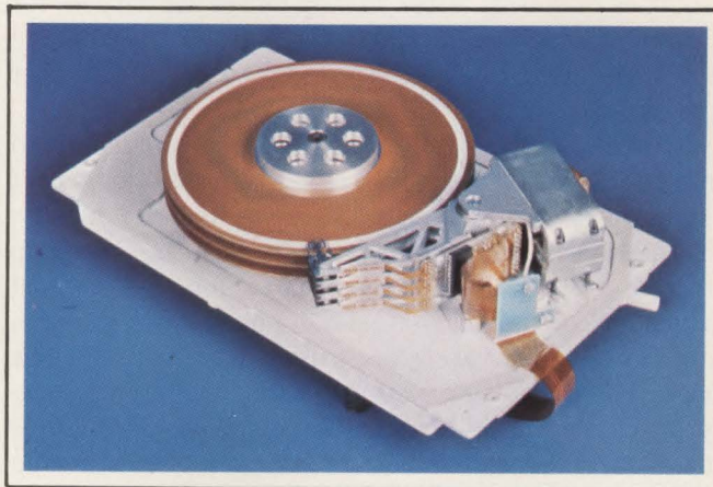
Track density is 172 tpi on Shugart's original SA1000 Winchester-disk drive and 500 tpi on the new SA1100.
