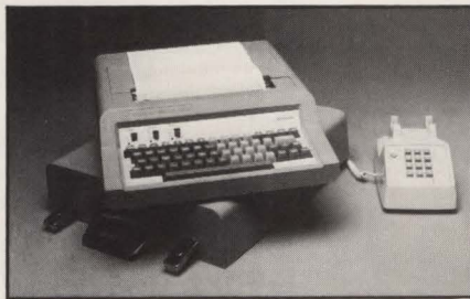
Using the "Comet" electronic-mail software package, Computer Devices, Inc.'s Miniterm portable terminal can access Tymnet, Telenet or direct-distance dial network.
