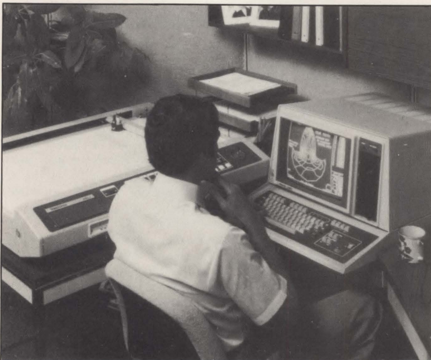
Tektronix's 4112 graphics display terminal is a monochrome raster display device that retains full 4010 software compatibility. It is priced at $9600.
