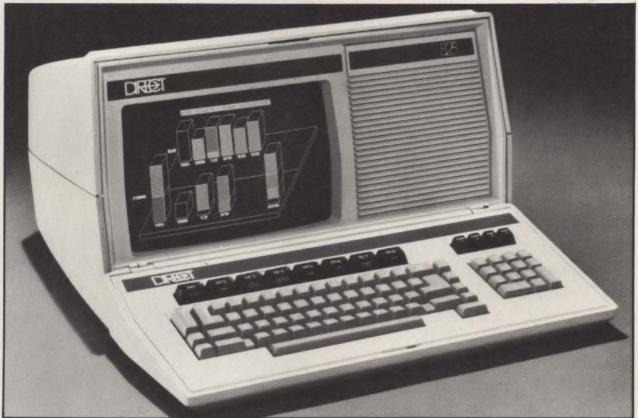
Direct's VP825 , an HP2622A-compatible device, uses H-P's View/3000 software, which handles screen-management and data-entry functions.
