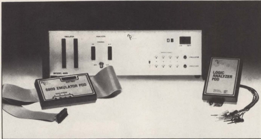
Advanced Digital Technology's model 4009 combines a real-time in-circuit emulator and a 12-/20-MHz, 18-channel logic analyzer into one instrument.
