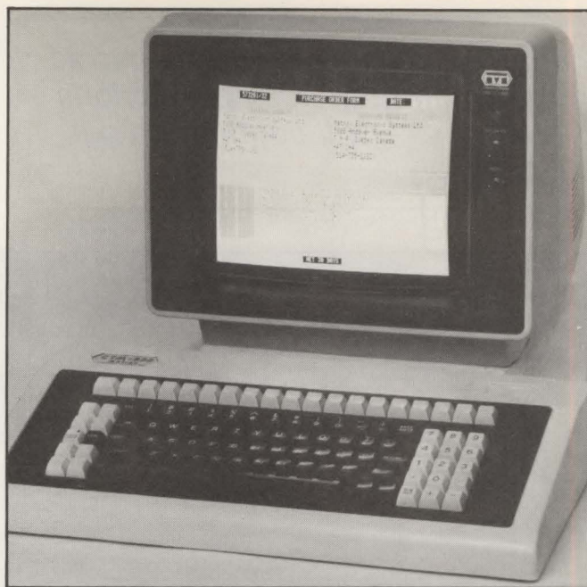
Matrox Electronic Systems' CTM-300 intelligent color terminal can be down-loaded from a host computer. The detachable keyboard has illuminated caps and shift-lock keys.
