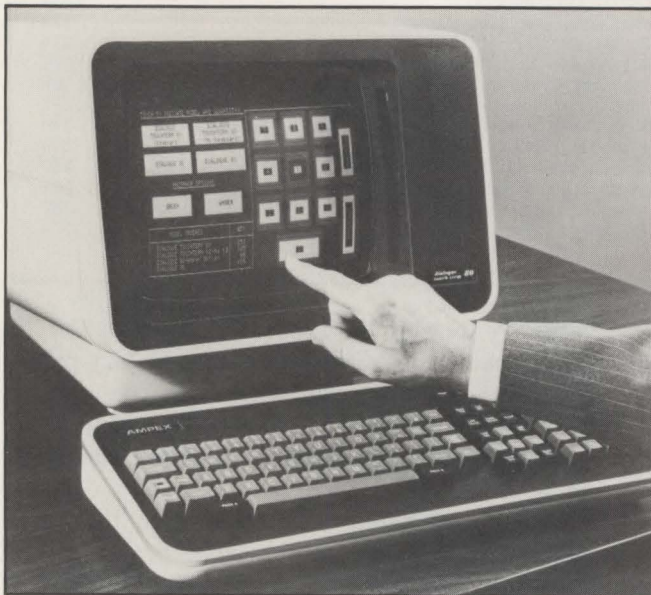
Ampex Dialogue Touchterm 80 editing terminal represents the latest effort of VDT manufacturers to boost capability beyond simple keyboard interaction. The Touchterm 80 uses scanning-infrared-beam technology for touch sensing. This allows not only soft-key (expanded keyboard) operation, but also stream-mode (digitizer) input of continuous-path and rate data.
