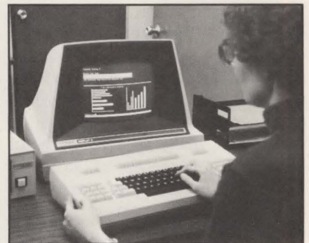
Computek's Display 8 terminal features a detachable keyboard with a 96 ASCII character set, 16 user-definable function keys, a 19-key numeric pad and 14 screen-management keys.
