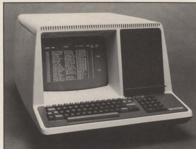
The VT52, one of DEC's VT50 series terminals, was considerably more versatile than the VT05. A boxlike cabinet and low-density circuit boards enabled cooling by natural convection. The VT52 featured both upper- and lower-case alphabets and an auxiliary keypad for numeric entry and cursor control. Adjustments for baud rate and line/local were made by using a screwdriver on recessed controls on the bottom of the terminal.
