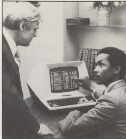
Burroughs's OFIS 1 office-automation system for professionals can be configured modularly to act as a word processor, an electronic file, a shared-resource system or an office-management system.
