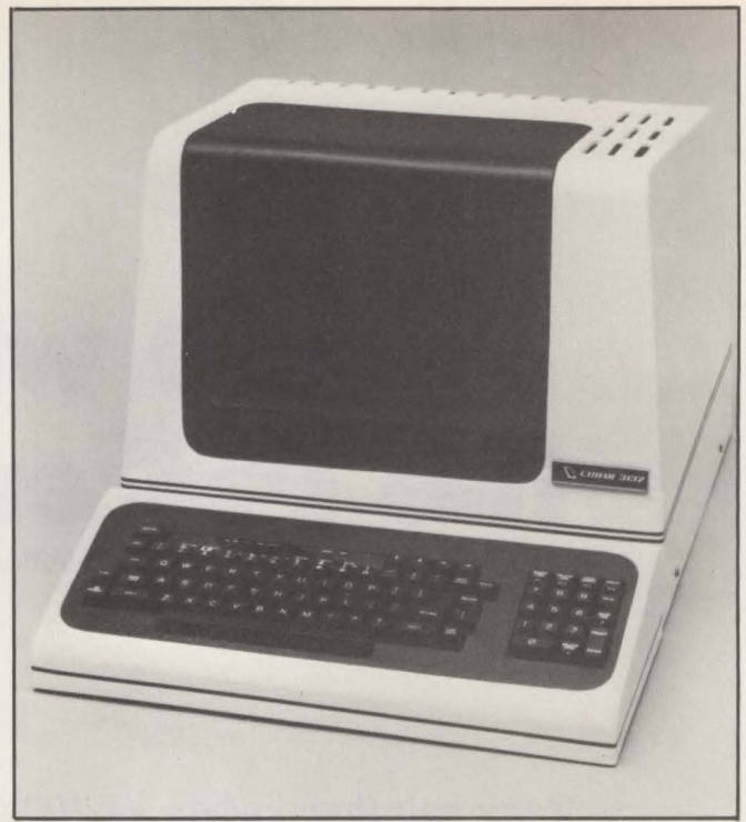
Cobar, Inc.'s model 3132 editing video terminal emulates DEC's VT-132, VT-100 and VT52.
