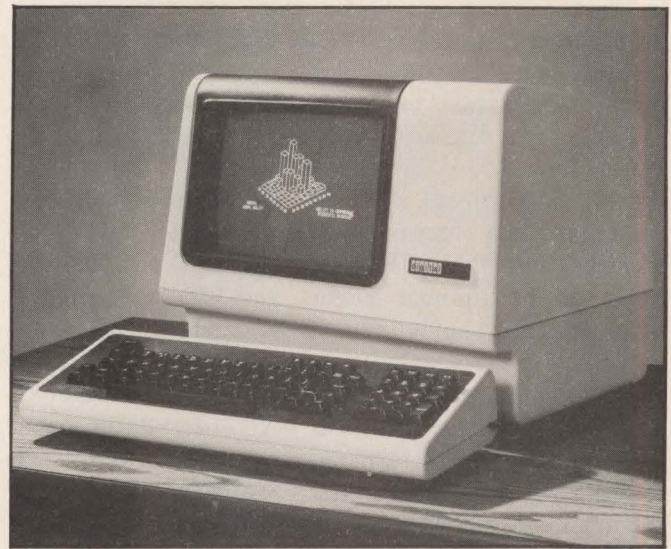
The addition of a graphics-board module converts DEC's VT-100 to the new VT-125, which allows images to be formed of individual dots rather than pre-defined 5 \times 7 matrixes.
