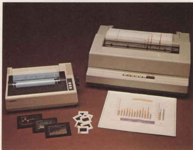
Hard-copy devices available for permanently recording ColorCalc/ColorGraph displays include black-and-white and color ink-jet printers (shown), color-slide cameras and cameras and images for off-the-screen or direct-from-memory Polaroids.
