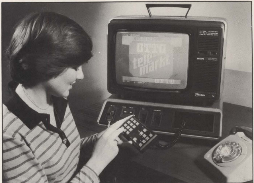
Through a new facility called Gateway, a private business computer system can be linked to a viewdata terminal using the pilot public viewdata service, Bildschirmtext, operated by Deutsche Bundespost, West Germany. British Telecom will add Gateway to its Prestel viewdata service next year.
