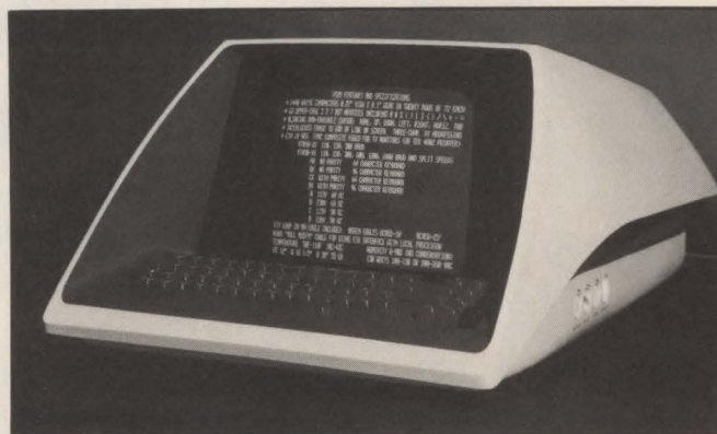
The VT05, DEC's first video terminal, is sculptured for aesthetics. The terminal used a conventional electronic design with closely packed circuit boards that required fans for cooling. Its character set included upper case only, and it did not provide for printers or equivalent satellite peripherals.
