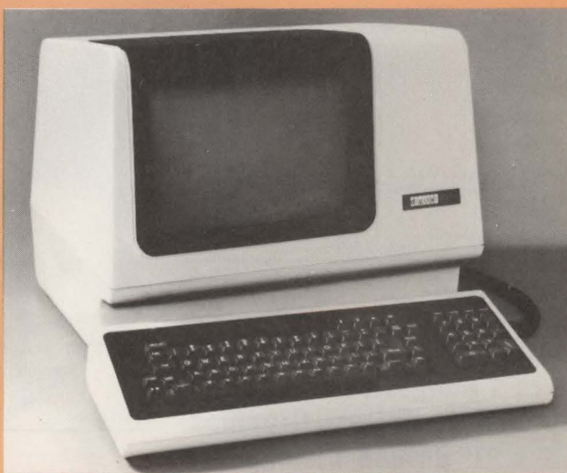
DEC's VT-100: The terminal that triggered all the emulation.
