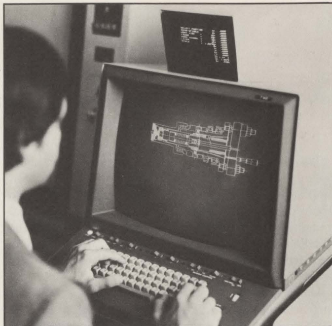
Fig. 2. McAuto's Unigraphics systems range in price from about $20,000 to $800,000 and can manage from one to 10 work stations. A total of 295 Unigraphics systems have been installed by McAuto worldwide to perform such applications as mechanical parts design and fabrication, pattern making, plastics-mold production and aluminum-extrusion die manufacturing.
