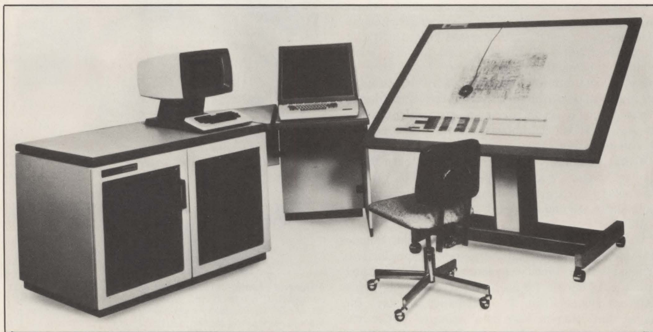
Fig. 1. Users claim 3:1 productivity gains with the Summagraphics Datagrid III computer-aided drafting system.
