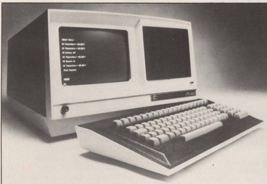
Codata's CTS-300 68000-based 16-bit \mu c can process FORTRAN and Pascal software, including FORTRAN-77, which previously could run only on mainframes or large minicomputers.
