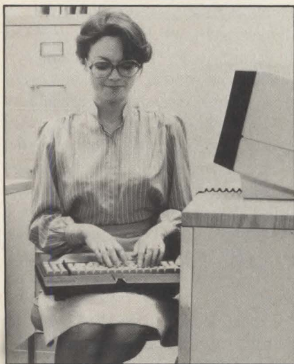
ADDS' Viewpoint terminal , designed for high-volume applications, offers a movable keyboard with numeric pad and sells for $650.
