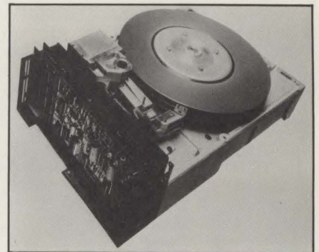
3M's 8533 Winchester-disk drive packs 60M bytes of data into a three-platter package the size of the industry standard SA850 floppy-disk drive.
