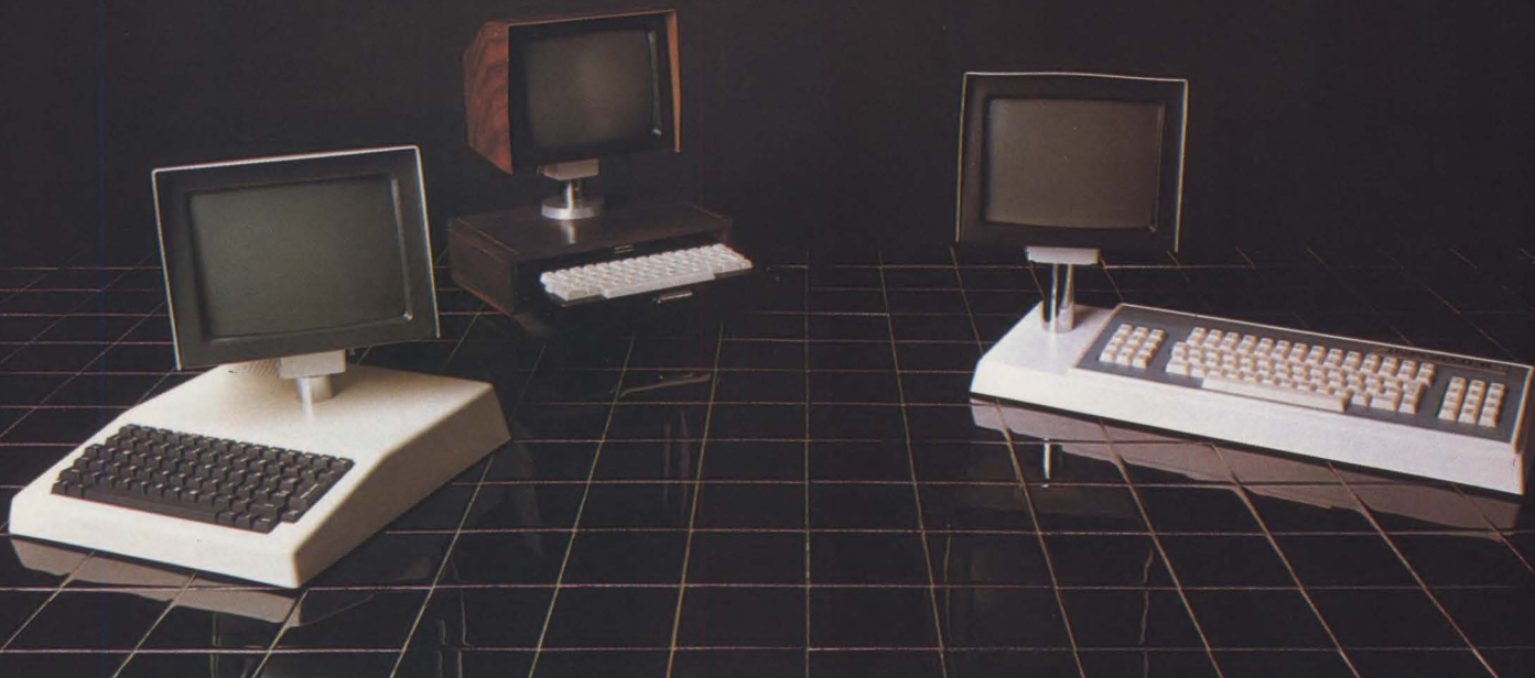
Model 401 Computer Terminal, 13" W x 14" H x 16" D, 14 lbs. Model I304 Data Inquiry Terminal, 13" W x 14" H x 13" D, 17 lbs. Model D304 Data Entry Terminal 26" W x 14" H x 11" D, 17 lbs.
