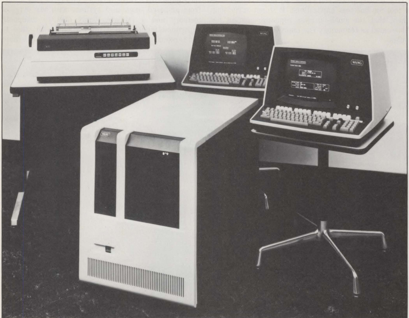
Wang Laboratories' 2200 LVP uses a 1M-byte, double-sided, double-density diskette and a 2M-, 4M- or 8M-byte fixed disk. User memory is expandable from 32K to 128K bytes.
