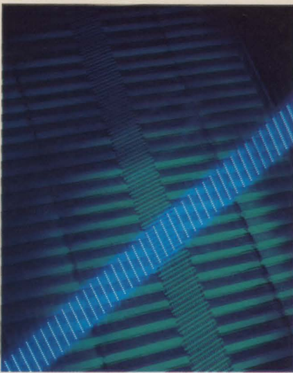
Circuit boards of Dephax's ion-cartridge "Otter" printer show holes through which ions are directed to print characters (see p. 179). Cover design and photo by Steve Grohe, Boston, courtesy of Delphax Systems.
