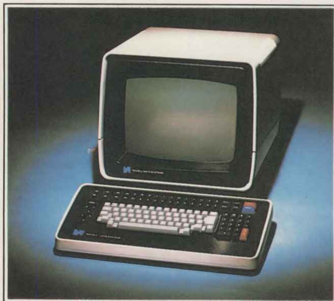
Novell Data Systems' Nexus II terminal computer is an 8-bit \mu c with 64K bytes of RAM. It includes the processor, memory, video display terminal and keyboard.
