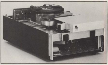
Pragma Data Systems model 2000 with cover removed shows proprietary ½-in. tape cartridge (foreground), immediately to the right of the rake-up reel. Read/write heads are mounted 180° apart in the drum to the rear. The entire package fits into the space required for an SA850 1M-byte double-sided floppy-disk drive.
