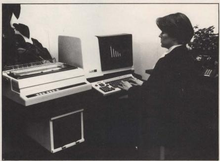
The Artelonics Series 1000 is the cornerstone of a family of management-information systems. Although it can be used as a word processor, it includes graphics, a CP/M operating system and the ability to program in Pascal.
