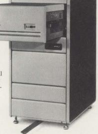
All air flow and electrical requirements have been integrated, so you need no separate air plenums or cable conduits.
