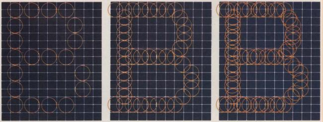
Fig. 4. The multi-pass technique "fills in" the vertical dots on each successive pass of the print head as the paper is moved vertically in a fraction of a dot-position.
