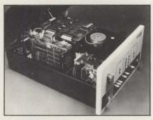
Xylogics's XL 2300 packaged μc system integrates an LSI-11/23 processor, 96K to 256K bytes of memory, Winchester-disk drive, cartridge-tape drive, eight RS232 ports and the support components required for operation in this compact cabinet.
