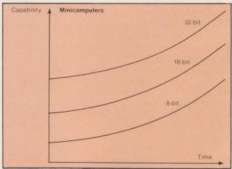
Fig. 3. Improvements in minicomputer capability are less dramatic because, as chips become more complex, some of their capability is lost to any particular application.
