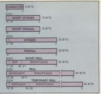
Fig. 2. The 432's hardware recognizes eight primitive data types.
