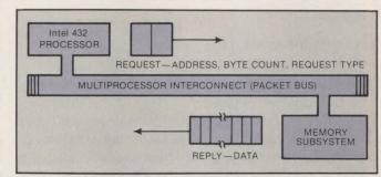
Fig. 1. The 432's packet bus can transfer as many as 16 bytes of data with a single request.
