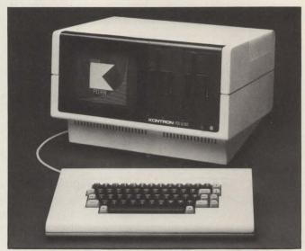
Using a Z80A  $\mu$ p, the Kontron PSI-80  $\mu$ c/controller supports foreground and background operations. It is designed for OEMs who require a system they can tailor to specific applications.
