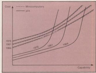
Fig. 1. Relative cost of minicomputer vs. µc operation: Micros are less expensive to use when the requirements are less demanding; more expensive when the task is more complex.
