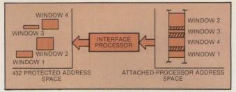
Fig. 7. An attached processor has access to main memory through windows that protect portions of memory not needed for the processor's operation.
