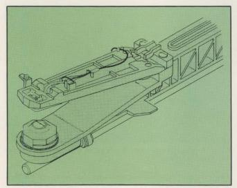
Fig. 2. New Bi-Compliant double-sided floppy technology uses a fixed lower head and a gimballed upper head.
