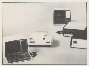
The dual Z80 µp-based WH-89 integrated machine (left) and the LSI-11-based 16-bit WH-11A systems come from Heath/Zenith either in kit form from the firm's Heathkit Division or assembled from the Zenith Data Systems Group.
