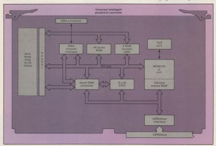
Fig. 5. As a specific example of an intelligent peripheral controller (IPC) board, this universal IPC block diagram illustrates the principal IPC components, including the interface to the high-speed system bus, the 8-bit μc unit with its dedicated ROM and RAM elements and "private" bus, and DMA controller elements to handle the high-speed data exchange.
