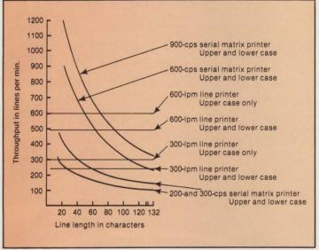
Fig. 3. Throughput comparison of serial matrix printers with 600-cps line printers.
