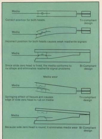
Fig. 3. If one of the head actuator carriage's flexures is bent at the wrong point, the head would not be parallel to the disk, causing media wear.
