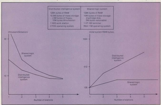
Fig. 5. Price and system capacity comparison between typical shared-logic and distributed-intelligence systems. As the number of stations increases, the price differential decreases, converging at about five stations. However, system capacity grows faster and more evenly in a distributed system, constantly matching resources to demand.
