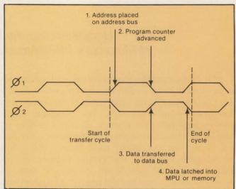
Fig. 2. Example of synchronous data transfer as used in 8-bit M6800-type μcs. A synchronized two-phase clock is distributed throughout the system and establishes the timing relationships for all data transfers.
