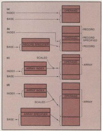
Fig. 5. Direct and indirect references can combine in four ways: Specify the index and base directly to access scalars (a), specify the base indirectly to access records (b), specify the index indirectly to access static arrays (c) and specify both the base and the index indirectly to access dynamic arrays (d).
