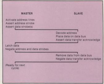
Fig. 3. Diagram illustrates the prescribed sequence of activities, or protocol, required to complete a single "memory read" transaction on a high-performance asynchronous bus, such as VERSAbus.
