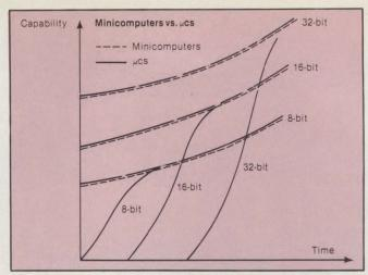
Fig. 4. Minicomputers start out with far greater capability than  $\mu$ cs, but improve less rapidly.
