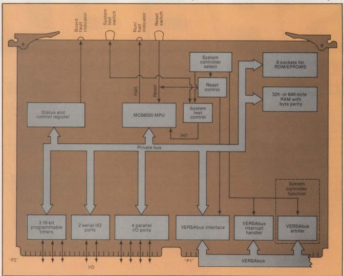
Fig. 4. Motorola's VERSAmodule monoboard μc offers a high degree of on-board 16-bit performance capability. The number of individual packages used (A) gives a clear indication of system design complexity, even with basic components of VLSI stature. Block diagram (B) illustrates functional capability.
