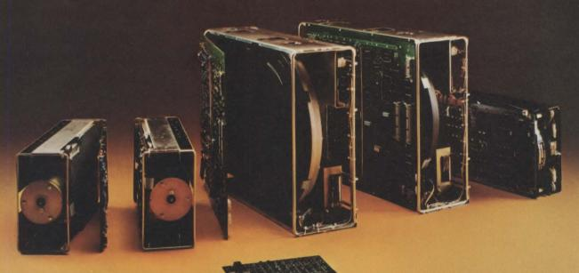
Members of this exclusive circle of PRIAM Winchester disc drives have several uncommon things in common. With database capacities from 10.8 to 158 megabytes, they all have the same interface. And they all connect quickly and easily to the typical microprocessor I/O bus through PRIAM's SMART Interface.
