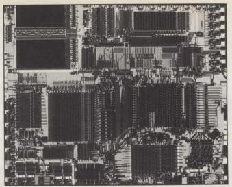
Intel's iAPX 432 micro-mainframe consists of three chips, which together house more than 200,000 devices. This is the 43203 interface processor.
