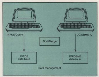
Fig. 2. Data General's data-management systems—INFOS II and DG/DBMS—each has an interactive query program, Query and DG/DBMS IQ.
