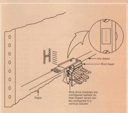
Fig. 1. Serial wire matrix printers operate by moving print head horizontally across the paper. Wires are configured in a vertical column and are selectively activated by wire hammer drivers to impact paper through an ink ribbon, thereby creating dot-matrix array characters on the paper.
