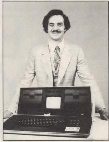
Adam Osborne and the Osborne I: Standard features of the new computer include two single-sided minifloppy-disk drives, 5-in. screen, Z80A µp and a foldup
