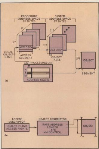
Fig. 10. Object addressing (a) in the 432 uses a contentsaddressable memory (CAM) as an address cache. It requires an access descriptor and an object descriptor that control all aspects of each object's manipulation.
