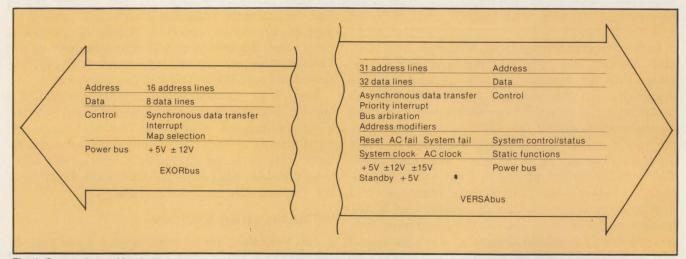
Fig. 1. Comparison of basic functions in a system bus serving the simpler 8-bit systems, and an advanced asynchronous bus serving higher performance 16- and 32-bit systems. The greatly expanded control functions of the 16/32-bit bus permit more efficient communications at a higher speed between independent computer elements sharing the common system bus.
