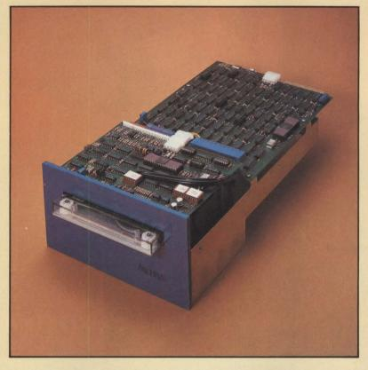
The intelligent Sidewinder handles tape formatting, error and file mark processing, tape positioning, automatic readafter-write error correction, block buffering and read
