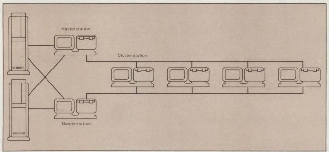
Fig. 4. Redundant master stations and mass storage increase the reliability of a distributed-intelligence system.
