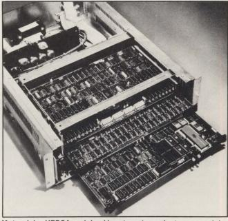
Motorola's VERSAmodule Monoboard μc features modular elements in a pre-wired chasses.
