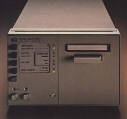
It's the HP 9915 Modular Computer — the first in a new generation of easy-to-use, low-cost computers for measurement automation.
