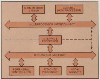
Fig. 6. A satellite subsystem (attached processor) can independently handle all I/O with the aid of the Multibus.
