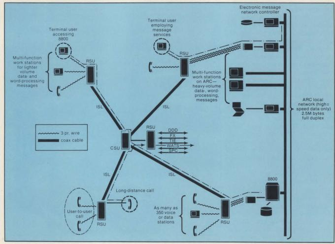
The Datapoint ARC and ISX combine to provide a high-speed data path and universal terminal access via RSU ports.
