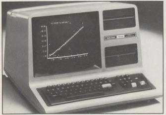
With two 51/4-in. floppy-disk drives and a full typewriter-like keyboard with upper- and lower-case characters, Radio Shack's TRS-80 model III replaces the firm's model I component system with a unitized package.
