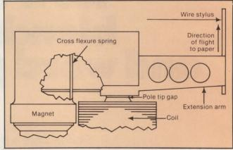
Fig. 2. Magnetic stored energy print head uses a cross-flexure spring held cocked by a magnetic field at pole tip gap. A coil is energized to cancel magnetic field of gap, releasing spring and allowing wire to impact paper at high speed.
