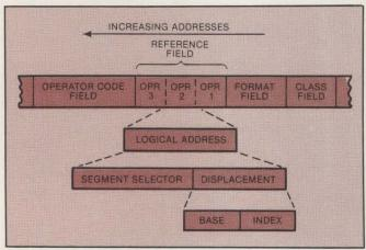
Fig. 4. Instruction-format length in the 432 varies and can accommodate as many as three operands.
