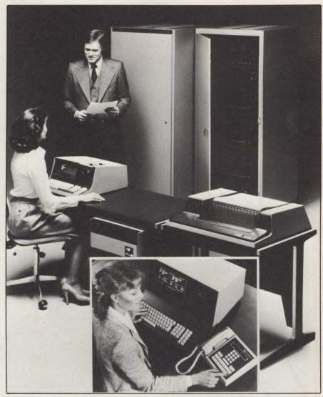
Datapoint's ISX is a digital PBX that uses dispersed switching technology to integrate voice, data, text, electronic message services and Datapoint's ARC coaxial cable local networks.
