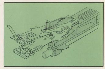
Fig. 1. Original tri-compliant double-sided floppy technology uses two gimballed heads.
