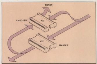
Fig. 9. Functional redundancy checking allows two iAPX 432s to check one another and flag computational errors.
