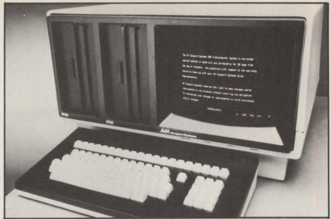
The J500 work station from AM Jacquard supports point-to-point or remote communications with the rest of the AM product line, including their high-quality phototypesetters.
