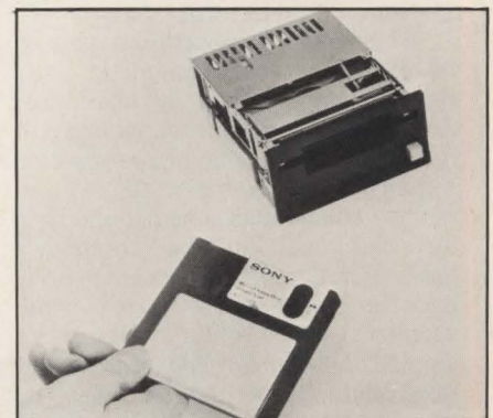
Sony's 3½-in. microfloppy-disk drive occupies 27 percent of the volume of conventional 5¼-in. disk drives, while doubling storage capacity.
