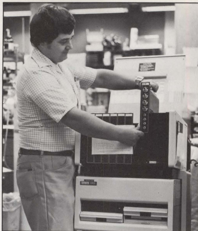
Klaus Liebold, computer director, inserts module in MINC system. Preamplifier, ADC, digital I/O and analog multiplexer modules can be interchanged to accommodate various experiments.
