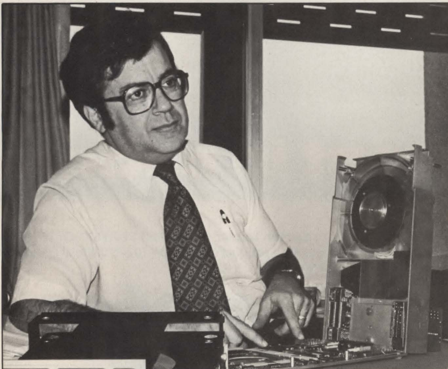
Perkin-Elmer's Don Friedman and a disassembled Vanguard 8C 8-in. Winchester disk-cartridge drive. View of the drive is from the bottom up and shows the "pancake" DC spindle motor.
