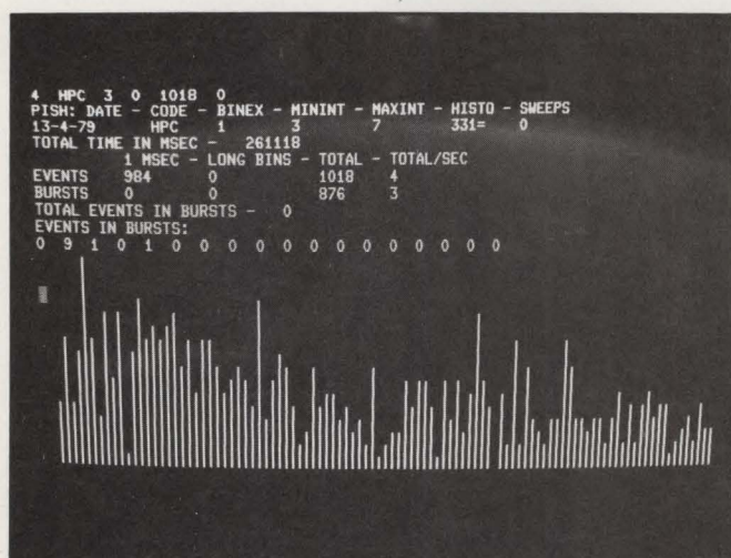
MINC has a command that causes post-stimulus-time histograms to be generated and displayed automatically, such as a frequency distribution of multiple brain signals against time.
