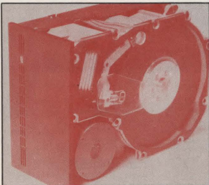
Computer Memories' CM 5000 —the highest capacity 5¼-in. Winchester announced so far—is in the final stages of development.
