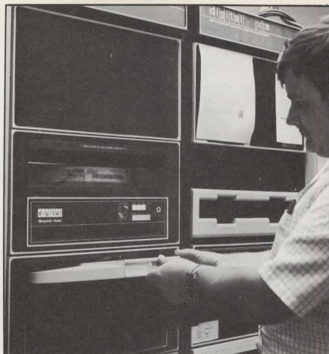
Klaus Liebold inserts a DECpack in the PDP-11/40, which is used to analyze data acquired on MINC system.
