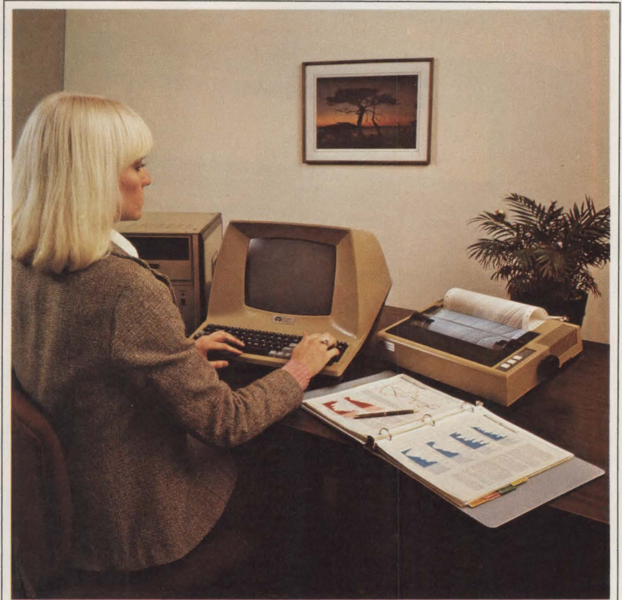
Monolithic Systems Corp.'s model 8802 software-development station includes a Multibus-compatible Z80A-based computer.
