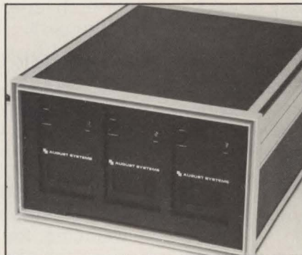
August Systems' BC 304 fault-tolerant computer "forgives" errors caused by electrical noise or hardware failures in industrial environments.
