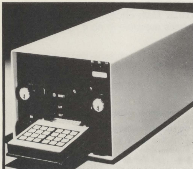
Fig 3. The Info-Guard data security system includes this network security module, which performs the NBS Standard. The complete Info-Guard key management system also includes a key generator and a key loader.
