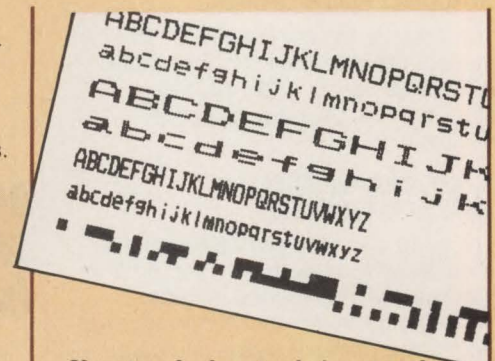
Unretouched, actual size samples of Microline printing. Standard, double width and condensed characters and 64 block shapes for charts, diagrams and illustrations.
