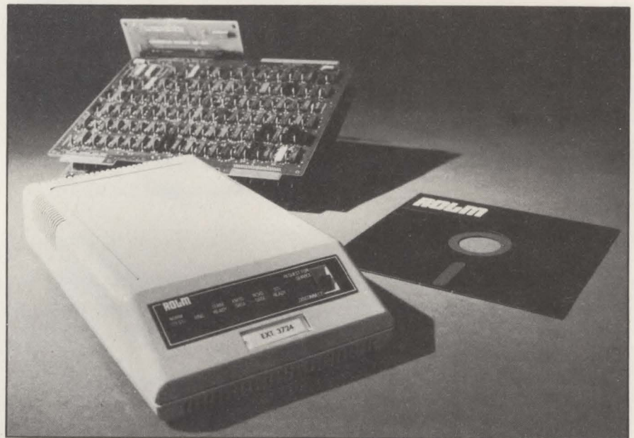
Rolm Corp.'s CBX, with a new data communications feature called submultiplexing, allows voice and digital communications between terminals, computers or other facilities.
