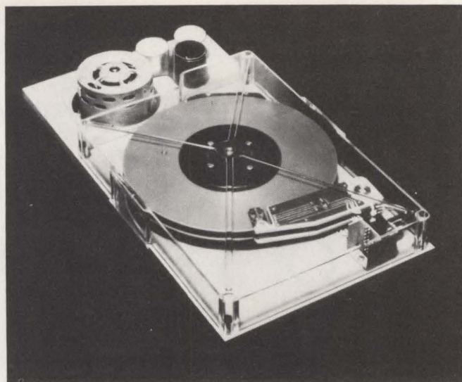
Fig. 5. The Kennedy Series 7000 8-in. disk has 5.5-MHz transfer rates and storage capacities as high as 20M bytes.
