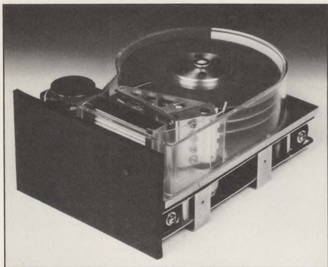
Shugart Associates' new line of 5 1/4-in. Winchester-disk drives offers as much as 10M bytes of capacity in a minifloppy-sized package.
