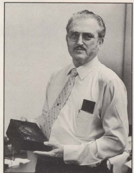
IMI's Al Hasler and the Series 5000 5¼-in. Winchester. The 7M-byte drive incorporates thin-film media and interfacing to Shugart's SA1000 8-in. device as well as to IMI's 7710, the first 8-in. Winchester announced for the OEM market.
