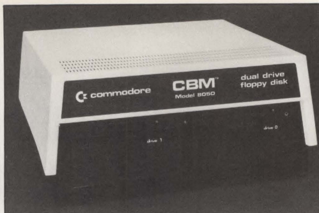
Fig. 3. Commodore Business Machines' model 8050 contains two 5¼-in. drives.
