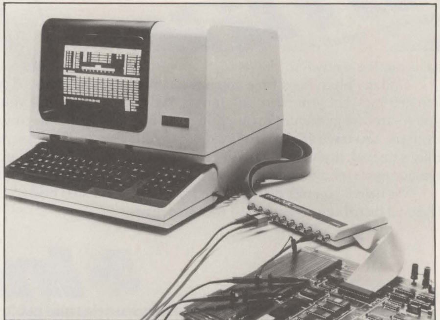
The Emulogic ECL-3211 is a 30-MHz universal emulation system that can operate as a stand-alone system or in a network with 64 stations controlled by a large host computer.
