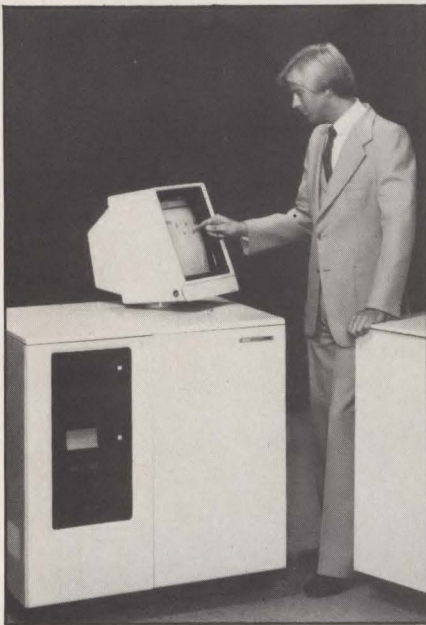
The 5700's touch screen serves as a control panel. A "help" button also is available to explain instructions to the operator.
