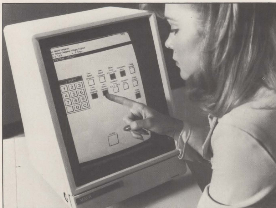
The Xerox 5700 printing system consists of two separate units: the touch screen and controller (left) and the printing system.
