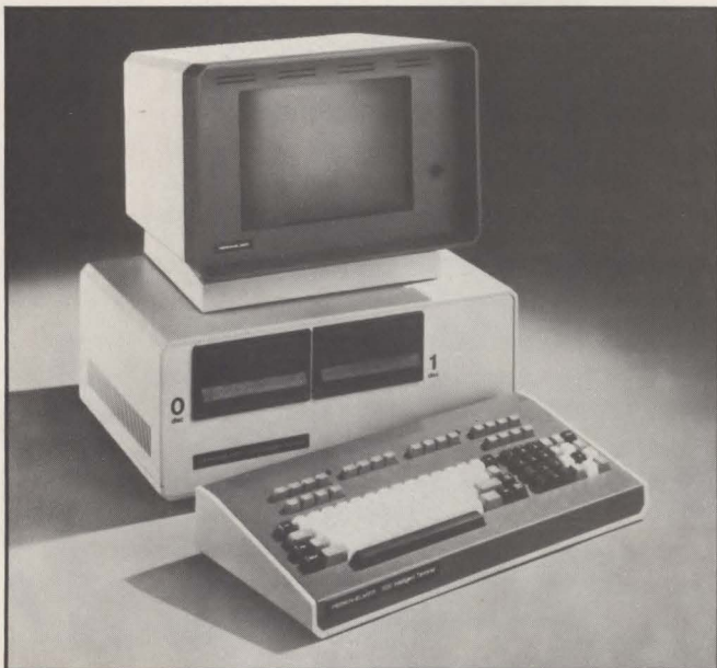
Fig. 1. The Perkin-Elmer model 3500 intelligent terminal with detached keyboard and dual floppy-disk drives.
