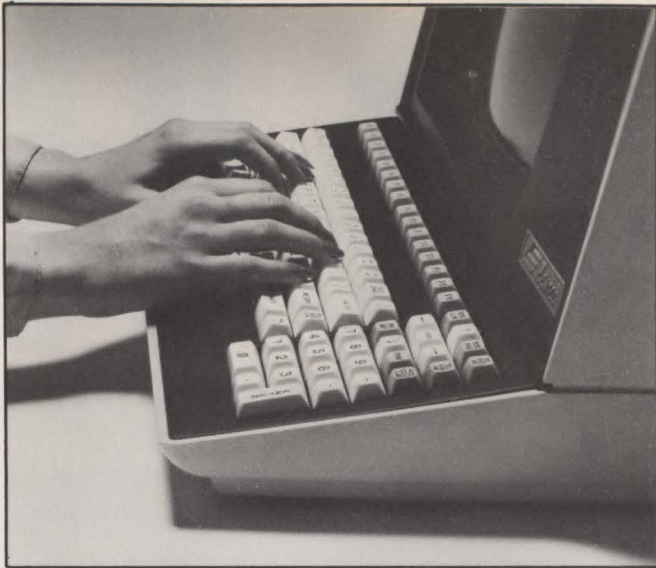
The stepped typewriter-style keyboard on the Zentec Zephyr (left) incorporates the standard 96 ASCII keys, a 14-key numeric pad, 12 special-purpose function keys and 16 programmable function keys. The ZMS-70 (right) has a similar keyboard, but it is detachable. The ZMS-70 also features a 15-in. non-glare CRT screen and dual, double-density, floppy-disk storage.
