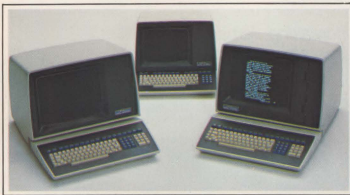
Zentec's ZMS-50 (center) incorporates a conventional attached keyboard with a 12-in. non-glare screen. The ZMS-90 (left) and ZMS-70 feature detachable keyboards and 15-in. non-glare screens. White phosphors are standard on all models, and green phosphors are available as options.
