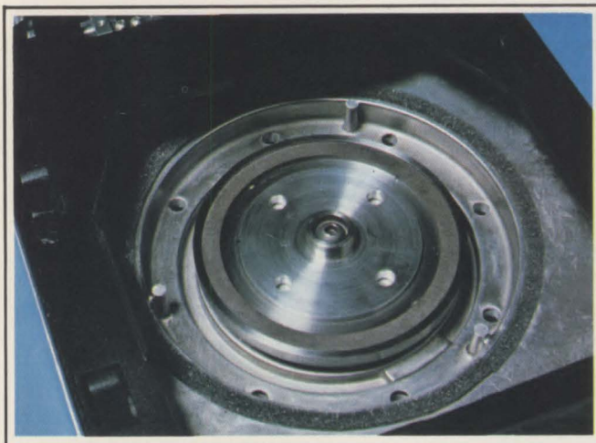
Fig. 3. Close-up of spindle and magnetic chuck. Cartridge's contact with the chuck frees the disk to rotate.
