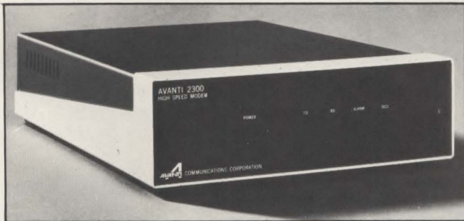
The Avanti 2300 modem is intended primarily for computer-to-computer and earth-satellite communication links.
