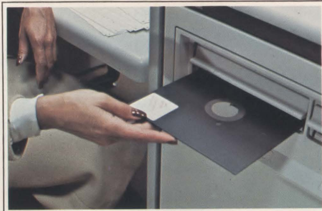
Model 9 includes one 1.2M-byte flexible-disk drive.
