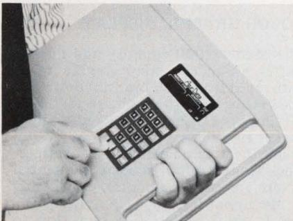
built-in battery pack provides for over 10 hours of operation. Standard memory is 2K, and is optionally expandable up to 12K. Price is \$1000 in single quantity. *Azur Data, Richland, WA.*
