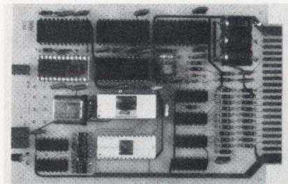
The input tones are split into upper and lower bands and filtered before being digitally detected. The module detects all 16 Touch Tone codes and provides for data storage and buffering. Optional buffering for up to 40 digits provides complete handshaking for direct connection to minicomputer or microprocessor data bus lines. Price is \$175 in quantities of 500. *BDI Electronics, Mountain View, CA.*
