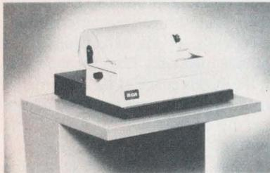
100 wpm. An optional eight-level ASCII version has speeds of 100 or 150 wpm. The teleprinter uses pressure sensitive paper instead of ribbon. A one-year lease is \$55 per month.
