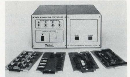
and software modules. Functions are defined in software so future changes can be made in the controller's PROM, not in hardware. Prices start at \$2500. *Tychon, Inc., Blacksburg, VA.*
