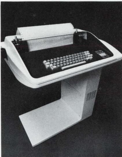
using a 96-character, upper and lower-case character set. Each character is formed by a 5x7 dot matrix. This version has as yet no provisions for paper tape or diskette for preparing data off-line. Initially Data General is going after its own customers and expects each processor system shipped will include a printer. (DG processor shipments averaged 5000 last year.)
