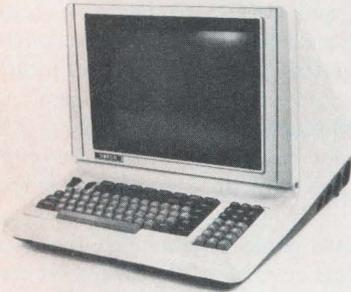
and stop/start bits. The 1920-character display uses a 7x9 dot matrix with half-dot shift for an effective 14x9 dot matrix. The unit is RS-232 or TTY compatible and communicates at speeds up to 9600 baud. Price is \$2750.
