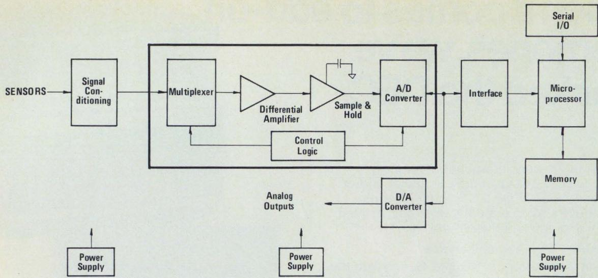
Fig. 3. Data Acquisition Module
