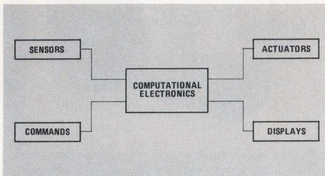
Fig. 1. Automotive Electronic System
