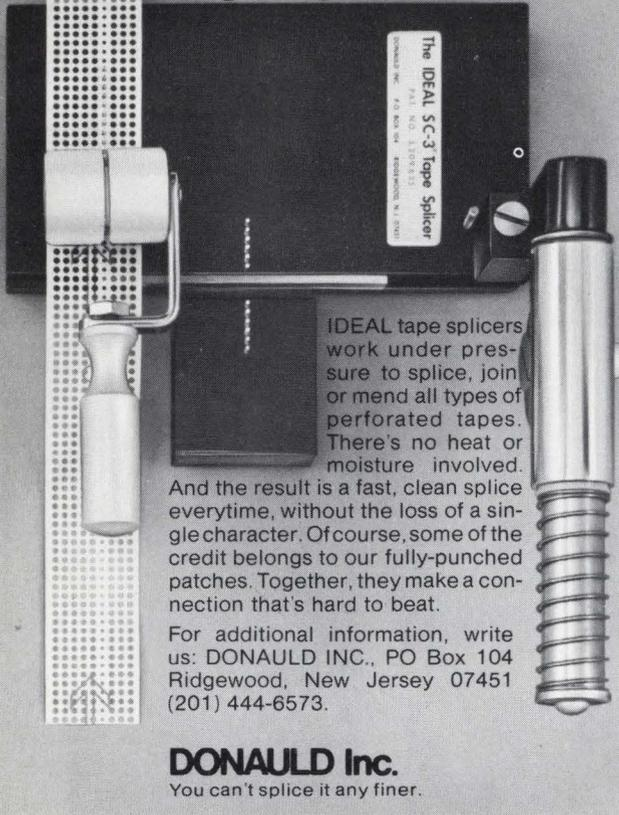
IDEAL tape splicers work under pressure to splice, join or mend all types of perforated tapes. There's no heat or moisture involved.
