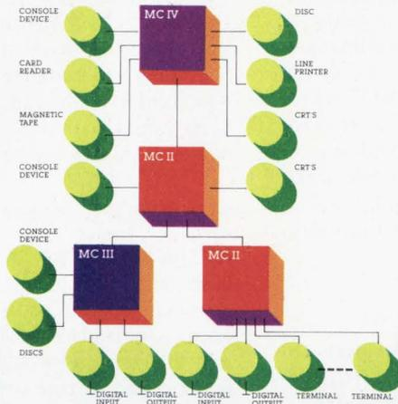
As the system has since evolved, a 32-bit MODCOMP IV now acts as host computer. Replacing (at a fraction of the cost) the company's former stand alone IBM 1800, the MODCOMP IV is expected to provide 10 to 25 times the throughput of the big machine, which had long since reached its saturation point.
