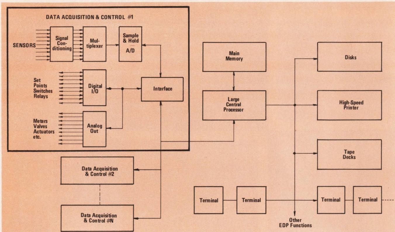
Fig. 1. Central Computer System With Data Acquisition & Control
