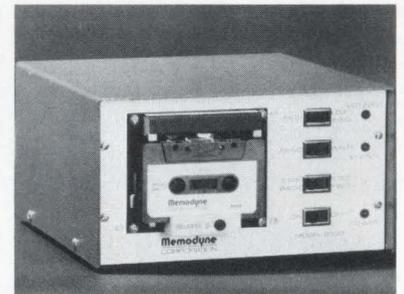
microprocessor-based applications, the recorder writes seven-bit ASCII or eight-bit parallel data using a standard Philips cassette. Price is \$775 in quantity.
