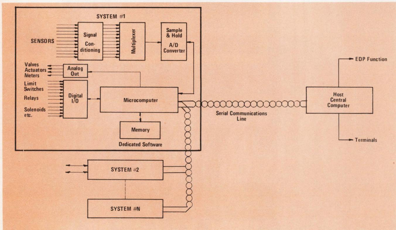
Fig. 2. Distributed Data Acquisition System With Microcomputer
