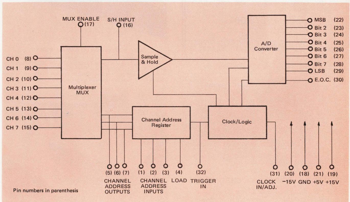
Fig. 1. DATA ACQUISITION IN 32 PINS. By using thin film hybrid technology, Micro Networks gets the major data acquisition function in one small package.
