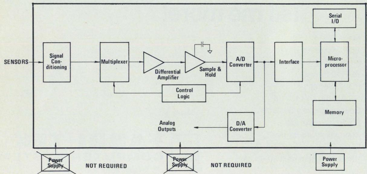
Fig. 5. Data Acquisition Computer
