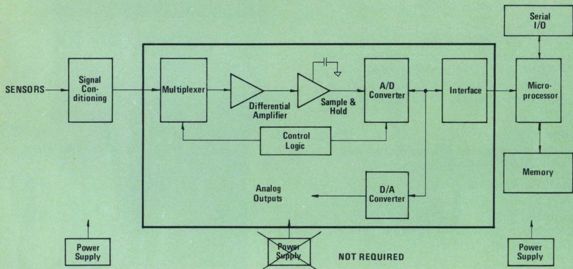
Fig. 4. Analog I/O Board For Microprocessors
