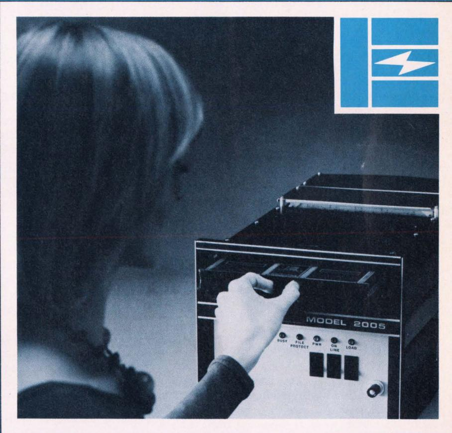
A standard Tape Pac® has 600 feet of 1/2-inch magnetic tape, (1000 feet optional), resulting in 12 or 20 megabytes of data storage. Basic transfer rate is 40K bytes per second.
