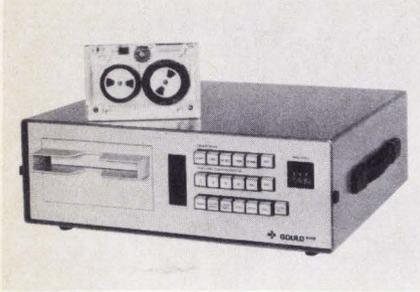
be all analog or up to 6 digital and 10 analog. Scanning rates are 1, 5, 10, 50, 100 and 200 points per second. Available output card options provide interfacing to most minis and programmable calculators, and an ASCII interface outputs data to any RS-232 teleprinter or CRT. *Gould Inc., Cleveland, OH.*
