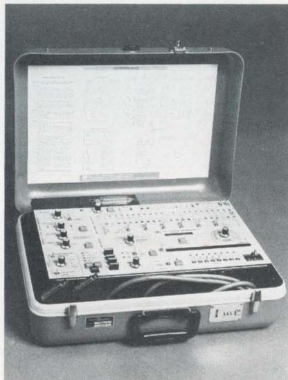
ing the calculation of block check characters. Intershake II offers the unskilled operator pushbutton selection of up to 15 protocol diagnostic routines. The skilled operator can structure these routines manually from a library of 100 programmable test steps including jump and branch instructions and loop instructions for software-like test programming. A CRT option allows simultaneous display of the full-duplex data stream, in clear text or hexadecimal.
