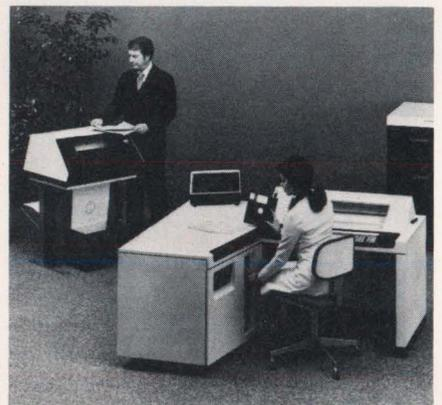
The performance of a B 80 basic system, with a 180 character-per-second console printer, is further increased by the addition of a 250-line per minute printer and two Burroughs dual-drive disk cartridge subsystems.
