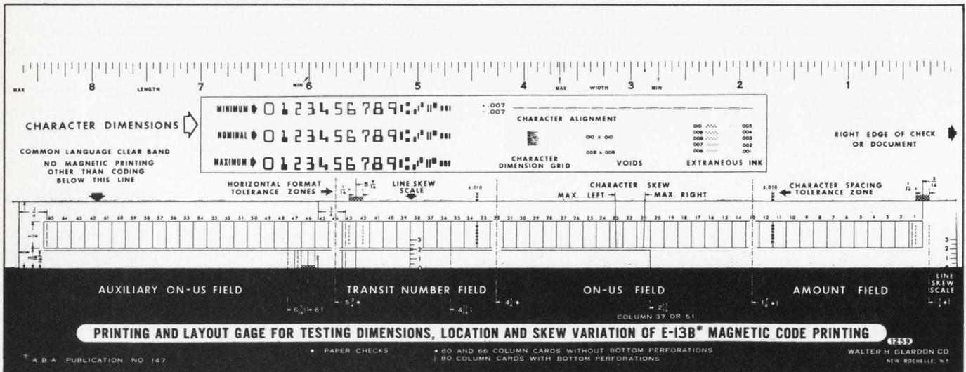
Fig 5 - Glardon gauge for alignment of MICR symbols on bank checks.
