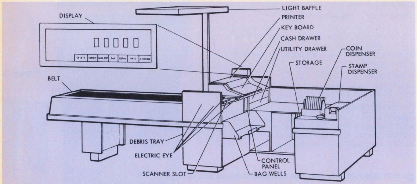
Fig. 1 — Schematic example of a POS checkout stand. (Courtesy of Sperry Univac)
