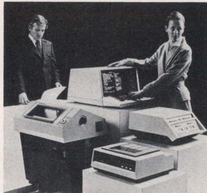
**UNIVAC'S INTELLIGENT TERMINAL.** The UTS 400 is a programmable, microprocessor-based display terminal which is compatible with Univac's Uniscope 100 and 200 communication procedures. Several peripherals can be added, including the Communications Output Printer, the Model 800 Terminal Printer and the Model 610 Tape Cassette.
