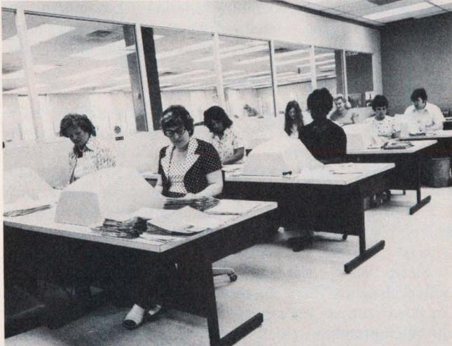
**KEY-TO-DISK IN ACTION.** An example of a shared-processor key-to-disk data entry system is the Entrex System 580 in operation at the VariTyper Division of Addressograph Multigraph Corp. With this Entrex System 580, department personnel at VariTyper have immediate access to a 2.5 million character Index Sequential Access Method (ISAM) master file containing information about all parts utilized in VariTyper's manufacturing process.
