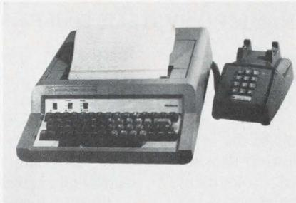
selectable keyboard, RS-232 interface and switch-selectable speed of 10, 15 or 30 characters per second. TI has a two-mode keyboard, optional RS-232 interface and a 90-day warranty. But perhaps most impressive about the Miniterm 1203 was that in showing the production process, a CDI engineer unassumingly snapped together the terminal in five minutes. That's modularity.
