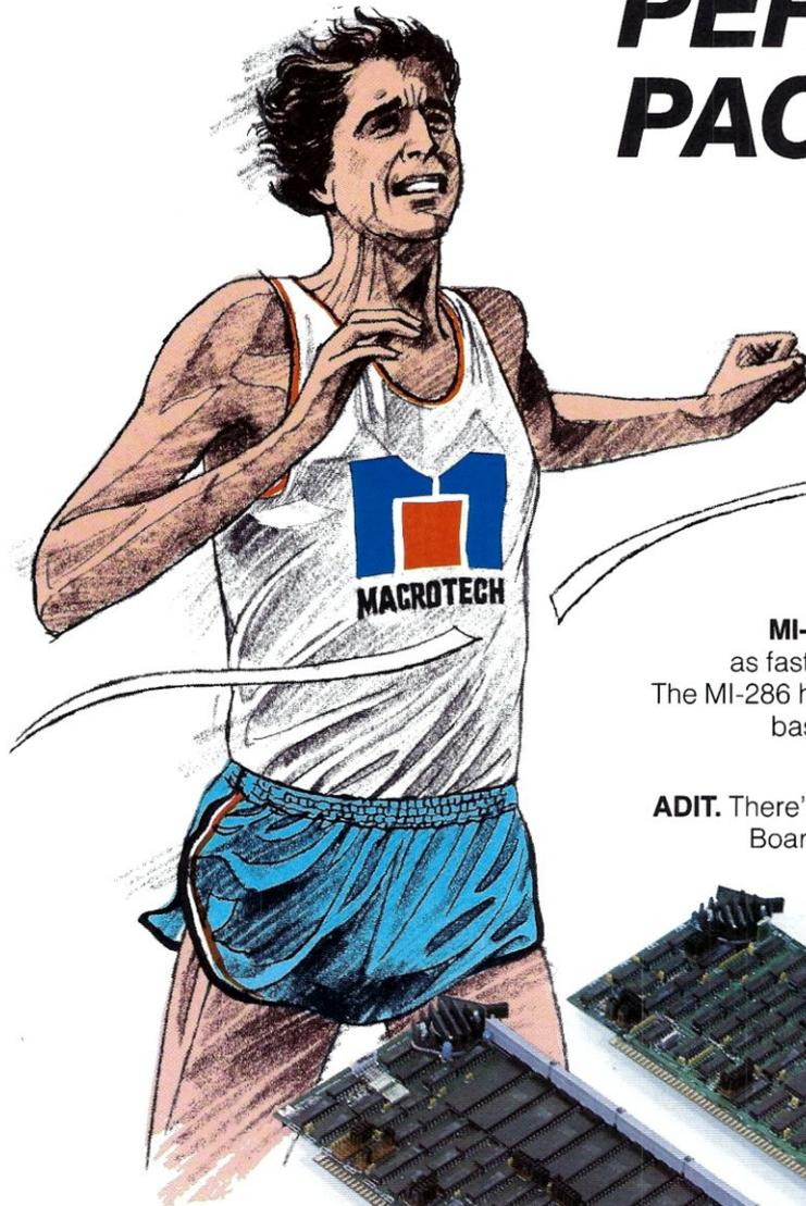
**MI-286.** Our 80286/Z80H Dual CPU Board is at least twice as fast as Compupro's 8085/88 and it's a direct replacement. The MI-286 has already become the standard by which other 80286 based systems are measured. Ask us for a complimentary Benchmark Report.
