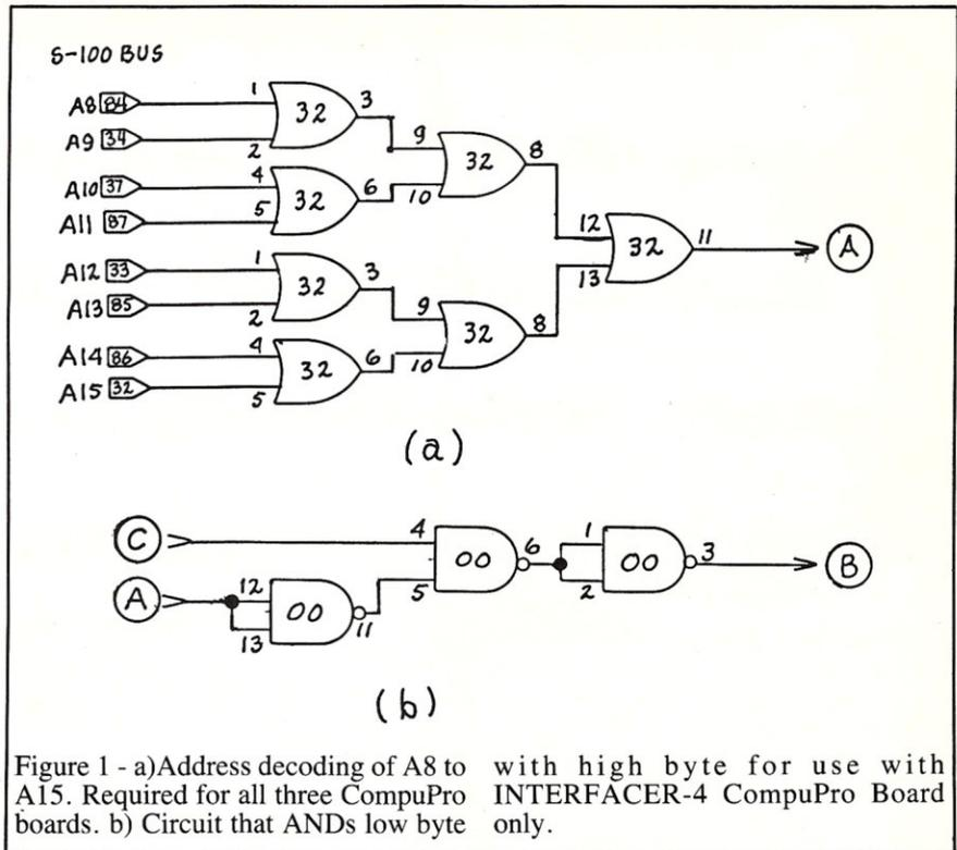
pin 3) on the board (Figure 1b). Instead of using two IC chips to accomplish this, a one package solution was to use several gates of a 74LS00. The address decoding output was inverted with one 74LS00 NAND gate, while two 74LS00 NAND gates were used to make the required AND gate. A wire soldered to pin 3 of U41 was used as one input to the AND gate (Figure 1 b). To complete the address decoding path, pins 2 and 4 of IC U23 were pulled out
