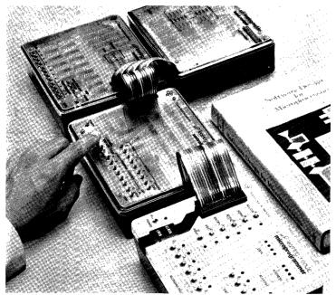
Each module has its own instruction manual, battery, charger and interconnecting cables and connectors. The system is provided with enough hardware and interface circuitry for the learner to design actual 4-bit applications.
