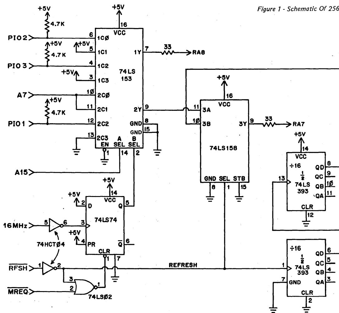
Figure 2 - Wiring Diagram For 256K Upgrade
