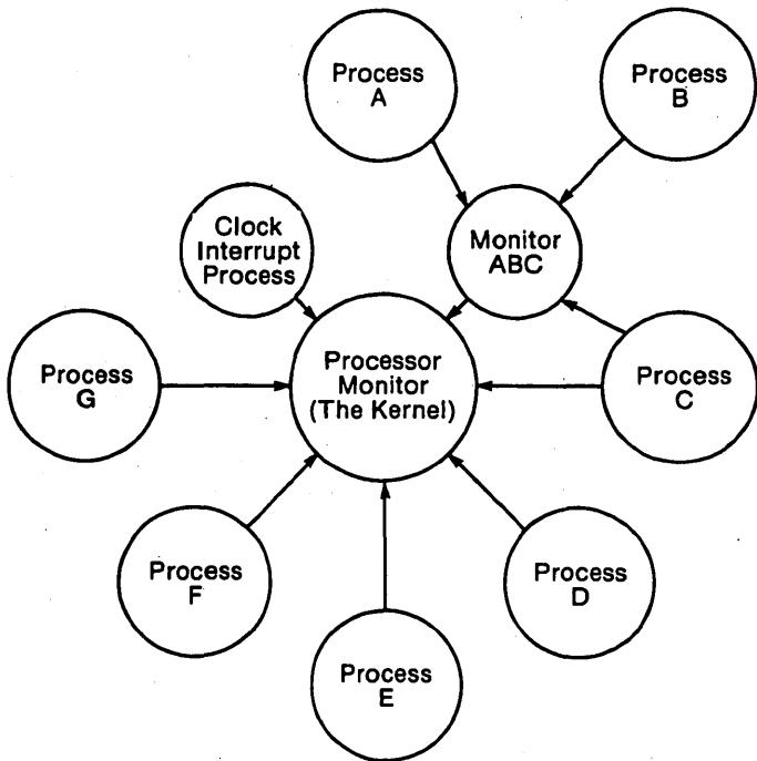
The clock interrupt handler provides the time slicing for the kernel. It knows when a process has used up its allotted time period. In this case the current process is preempted if any other processes are in the Ready queue. This interrupt handler also provides the mechanism for managing the Sleepqueue.
