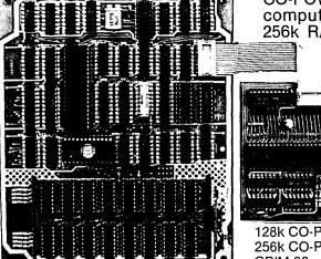
CO-POWER-88 is a 16-bit 8088 coprocessor for Z80 CP/M computers. Both versions of CO-POWER-88, 128k and 256k RAM, include both MSDOS, and RAM drive software, complete with MSDOS, IBM-PC compatibility.
