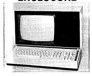
12" Green Ball Brothers monitor with enclosure measuring 19" × 16.5" × 14". Room inside to mount a Ferguson single board computer or small SS-50,S-100 system. (Power supply available, see below.) Requires +15 volts DC. @ 1.5 amps, noncomposite (separate sync) input. A sync separator schematic is available. It is also possible to mount a single 8" disk drive or two of the new slim line 8" disk drives in this enclosure. All units are used, and have been 100% tested.
