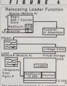
The source for program A is compiled and transformed into object code. The MVS Linkage Editor reads the object code and creates a load module. The initiator loads program A, which causes the contents of program A to be altered based on the point in virtual storage where program A is loaded.
