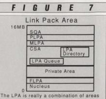
built by MVS as it is initializing and control blocks which hold pointers to the modules.
