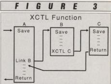
In MVS, one module can transfer control (XCTL) to another module. In this example, module A has linked to module B, but in module B it is determined module C must finish the process. AN XCTL macro is issued with loads and transfers control to module C. Return is back to module A.
