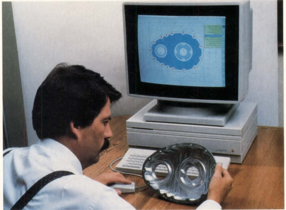
Figure 2—A Macintosh II running MGMTStation CAD/CAM software provides a powerful engineering workstation for a host system.
