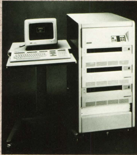
The Archeion, EMC's optical disk storage subsystem, provides up to 56 Gbytes of online storage for VAX users.
