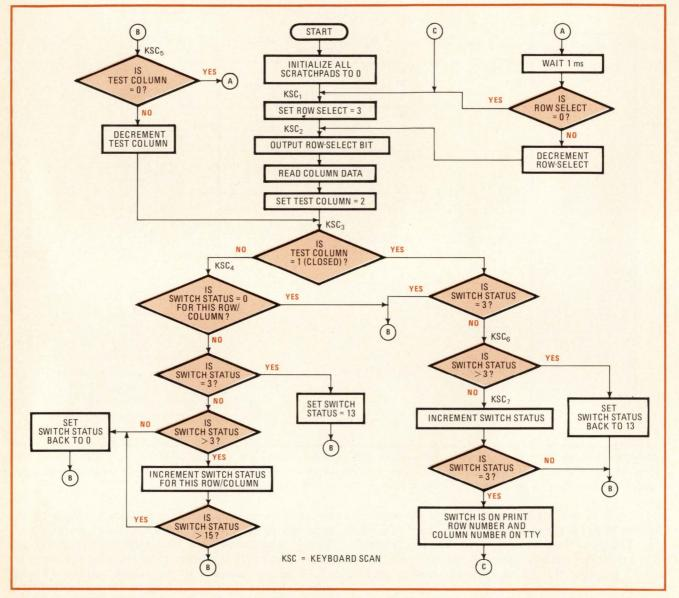
**4. Scan routine.** The F8's decisions and timing required for software sensing and debouncing of the 4-by-3 switch matrix proceed as shown. The KSC<sub>N</sub>, KSC<sub>N</sub>, KSC<sub>N</sub>, KSC<sub>2</sub> symbols are the keyboard scanning intervals used to sense the condition of a particular switch.
