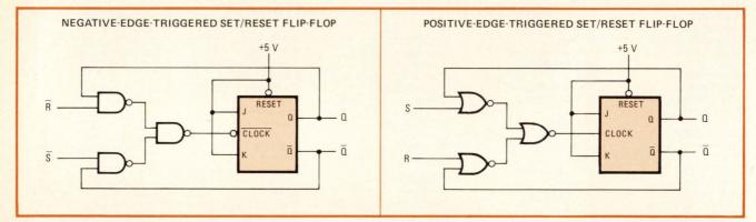
**Getting the edge.** Negative- or positive-edge-triggered R/S flip-flops can be made by adding NAND or NOR gates to a J-K flip-flop. The flip-flop at left must be negative-edge triggered, like the 7473, while the unit at right must be positive-edge triggered, like the 7470.
