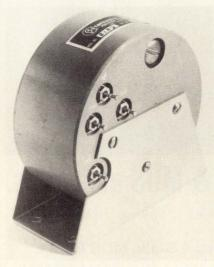
The mechanisms are hermetically sealed in silicone oil, which acts as a damping medium. Various oil viscosities may be specified to provide the damping characteristics required by a particular application. Pendulum potentiometers are available with diameters of 2.5 and 3.0 inches. Pendulum Pots, Betatronix Inc., 100 Ricefield Lane, Hauppauge, N.Y. 11787. Phone Joseph J. Yanosik at (516) 543-8780 [376]
