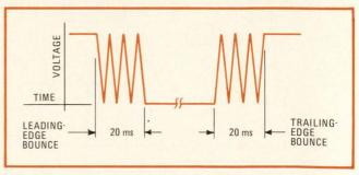
2. Switch bounce. Mechanical key switches have more than one closure upon actuation or release. Ordinarily, RC filters are used to minimize bounce, but the F8's software scanning technique filters bounce by taking multiple samples of the switches' conditions.
