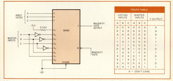
2. Veto power. Adding a few inverters to the circuit provides it with master-override capabilities. Whichever input is selected as master, the output always agrees with the vote of that input, regardless of the votes of the other two.
