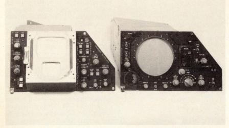
**New view.** Engineering model of the F-111F's new sensor display, left, fits two cathode-ray tubes into the space usually occupied by one circular display, right. GE's virtual-image magnification system would fit over and enlarge the twin CRT images.
