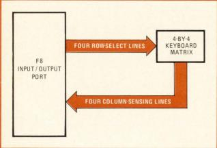
**1. Scanning the keys.** With one F8 port, a 16-switch keyboard can be scanned with no external hardware. The bidirectional property of the F8 microprocessor's I/O ports makes this possible.
