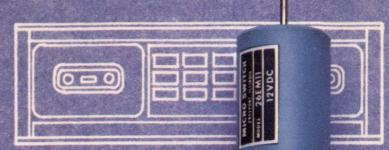
IDEALLY SUITED FOR DIGITAL CASSETTE RECORDERS AND CARTRIDGE DRIVES, THE 26 EM MOTOR USES A HOLLOW ROTOR TO PROVIDE THE LOWEST POSSIBLE ROTOR MASS RESULTING IN VERY LOW INERTIA. DIRECTLY INTERCHANGEABLE WITH MOTORS MADE OUTSIDE USA.
