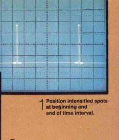
Switch to delayed sweep mode and use  $\Delta$  Time dial to superimpose beginning and end of interval.
