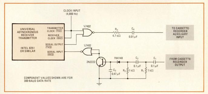
Easy interface. Far simpler than frequency-shift-keying systems, this computer/cassette-recorder interface does not even need a tone generator — the clock to the universal asynchronous receiver/transmitter provides it with a tone, which is gated on and off.
