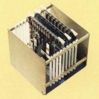
Both cards are easily interfaced in a simple, low-cost card cage.
