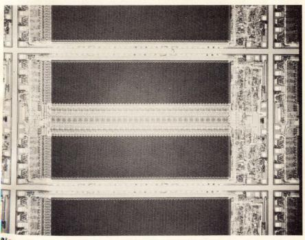
**Big and fast.** This Mostek 16,384-bit RAM is fast and dissipates low power because of a tight WO-level polysilicon cell design and sense amps that use power only when sensing.
