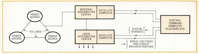
**5. Power generation.** Monitoring, managing, and control of a power grid is best done by a distributed network. A typical system will have a number of regional centers and associated local centers, all with processors tied into the central computer.
