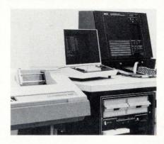
unskilled operators to isolate circuit-board faults. System hardware includes a 16-pin IC clip and a single-tip probe. Connected by cable to the 6500 test head, the clip and probe are positioned by the operator in accordance with instructions displayed on a CRT terminal. Both clip and probe are protected against overvoltages to ±30 volts.
