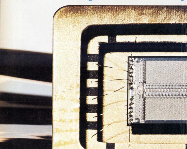
RAM — goes through an arduous series of screens and stresses: Full parametric preburn-in testing. Temperature cycling. Centrifuge. Dynamic burn-in at 125°C. And final test at high temperature with wide guardbands. Want proof? Ask our customers.
