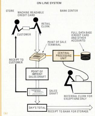
**6. Electronic credit.** Credit-card transactions can be made by the off-line method, top, or the on-line method. On-line authorization uses an intelligent point-of-sale terminal as the remote processor of an overall distributed-control system.
