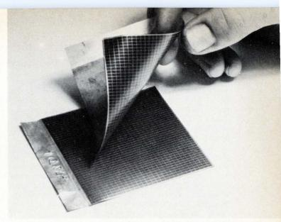
**2. Next generation.** Least expensive of photovoltaic materials, cadmium sulfide has a theoretical 20% conversion efficiency. These thin-film CdS cells, developed at the University of Delaware's Institute of Energy Conversion, have attained 7.8%, the highest yet.
