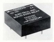
switch up to 3 amperes at 120 or 240 volts ac. Versions are available with input-voltage ranges of 3 to 8, 8 to 18, and 18 to 32 v dc. Capable of being driven directly by TTL levels, the relays offer zero-crossover switching and optical isolation between input and output. The price is \$5 each for 1,000 of the 1.5-ampere 120-volt version, and \$5.79 for the 3-A 120-V unit. Delivery time is six to eight weeks.
