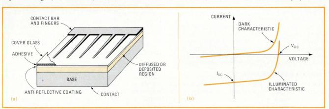
1. Typical solar cell. Essentially, a solar cell is a semiconductor photodiode. It is made up of seven structural elements (a), starting with a base contact and topped by a cover glass. Electrically (b), it behaves like a conventional junction diode when not illuminated. But when illuminated, it develops a small electrical signal, even though no external bias voltage or current is applied.
