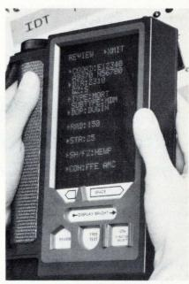
**Clear view.** Message keyed into interactive display terminal via transparent switch over light-emitting diodes (left) is reviewed for accuracy before being transmitted.
