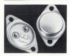
overload protection. If the junction of the power output transistor gets too hot, the regulator simply shuts down before it damages itself or any other system components. The 78H05KC is available from stock.
