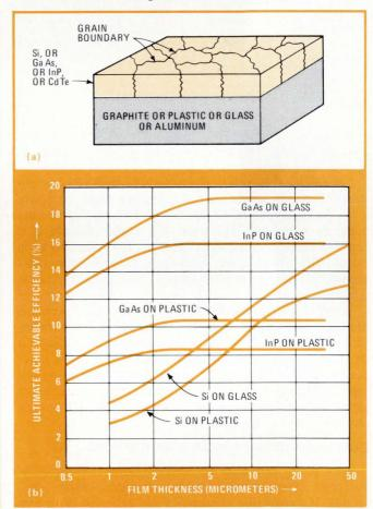
**5. Low cost but not yet practical.** Solar cells (a) made with thin films of polycrystalline semiconductors on inexpensive substrates hold the promise of reasonable efficiencies at low fabrication costs. The curves (b) show the theoretical efficiencies achievable for various combinations of substrates and semiconductor films, as a function of the thickness of the semiconductor film.
