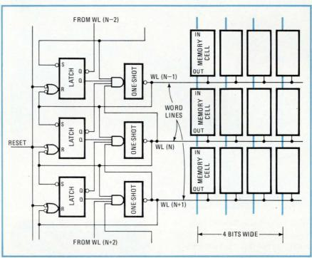
**Shift down.** Control circuitry for the 67401, comprising latch, AND gate, and one-shot, monitors cell contents and allows data to propagate from top to bottom. Data does not shift from word-line N-1 into N unless the line is empty, having sent its contents to N+1.
