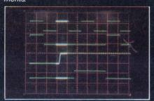
Here the main and delayed timebases are triggered from different channels, one example of the PM 3244's unique triggering facilities. Signals can therefore be shown even when they are not related to the main timebase.
