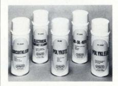
moves solder flux and other residue from printed-circuit boards, Polykleen is a fast-drying degreaser, and Electrical Contact Cleaner is just that. Polykote is a polyurethane lacquer for touching up and repairing printed-circuit boards and damaged insulation. And No-Sil-Kote is a silicone-free, paintable, mold-release agent, which is nonflammable, nonoxidizing, and greaseless. All five materials are packaged in aerosol cans and bulk containers.
