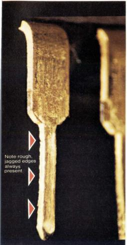
Your IC lead frames look like this at 30X enlargement (unretouched). Because they are punched out of metal, the edges are rough, jagged and irregular. In contrast, the flat sides of the lead frame are smooth, even and perfectly plated.
