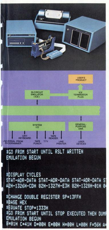
The Intellec system includes its own 8080 processor, memory, and a full range of peripherals designed to ease your development task. These include diskette operating system, CRT/keyboard, line printer, universal PROM programmer, high speed papertape reader, the in-circuit emulation modules, (ICE-80 and ICE-30) and interfaces for teletypewriter and high speed tape punch.
