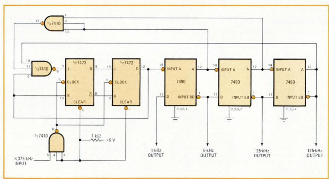
**Frequency divider.** This circuit uses a dual flip-flop and three divide-by-2 stages with feedback to divide the input frequency by 27. Three divide-by-5 stages then give further reductions. The input frequency of 3,375 kHz is convenient for use as a laboratory standard oscillator frequency because it has many useful submultiples and, besides, can be calibrated with great precision simply with a color-TV set.
