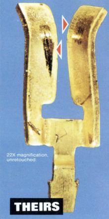
An ordinary edge-bearing socket contact after 5 insertions of DIP lead frame. Contact has been spread apart to show inside faces of contact. Notice how the contact has scars and abrasions from rough, irregular edge of IC lead frame. Electrical contact is degraded and resistance is increased. Reliability is obviously reduced.
