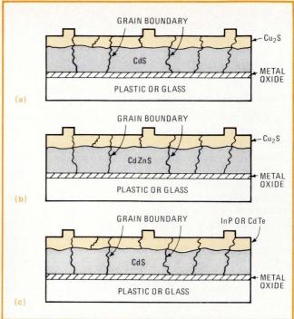
**3. Cadmium sulfide for low cost.** Although they deliver efficiencies of around only 6%, CdS solar cells are cheapest. They can be built on inexpensive substrates, like plastic or glass, with a cuprous-sulfide coating over either CdS (a) or cadmium zinc sulfide (b), or with either indium phosphide or cadmium telluride over CdS (c).
