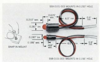
558 and 559 SERIES Available with  $6^{\prime\prime}$  wire leads, these red, green or yellow LEDs are designed for quick positive insertion in 0.031" to 0.062" panels. Compact design allows high density packaging. In 1000-lot quantities each
