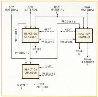
Distributed system. Because all the three chambers used in this process are interdependent and remote from each other, the system can be classified as distributed.
