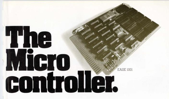
Just plug programmed PROMs or one 16K ROM into the EASE 1001 board to make an operational microcontroller. Excellent for prototypes—and the final product in many cases.
