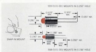
558 and 559 SERIES Available in red, green or yellow LEDs, with and without integral current limiting resistors. Snap-in mounting requires no additional hardware. Straight terminals suited for wirewrapping and/or soldering. Low power requirements— 15 to 20mA. In 1000-lot quantities each
