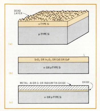
**2. Good efficiency with silicon.** Solar cells based on Si provide reasonable efficiencies—on the order of 15%—at reasonable cost. Several variations look quite promising—among them nonreflecting (a), heterojunction (b), and Schottky-barrier (c) structures.
