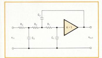
**1. Uses loose-tolerance components.** The performance of this three-pole low-pass active filter is insensitive to values of resistors and capacitors if the amplifier gain, K, is unity. Therefore inexpensive components with relatively loose tolerances can be used.
