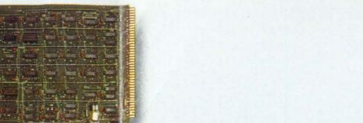
**I/O Distributor.** Model 14629-XX. In conjunction with Intelligent Cables (see text), the I/O Distributor provides up to eight interfaces—serial or parallel in any mix. Small version accommodates four interfaces. A DMA version allows data transfer rates up to 250K bytes per second.
