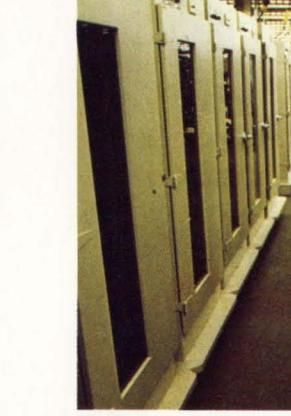
Temperature chambers stress computers to isolate marginal components. Computers are continuously tested during 72-hour burn-in at 50°C. Any error starts the test over from the beginning. To further stress the computer, power is cycled on and off approximately 2000 times during test.
