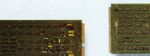
**Synchronous Modem Controller.** Model 14513-00. Double buffered, half or full-duplex interface for synchronous communications line (point-to-point, multipoint, or direct dial). EIA RS232C/CCITT compatible, programmable synchronous character, and one special character detect. Odd, even or no parity and 5-8 bit frame size program selectable. Transfer to 9600 baud.
