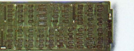
**NAKED MILLI LSI-3/05 CPU, Type 0.** Model 10300-00. Small low-cost processor offers exceptional power and features. 95 instructions, Power Fail Restart, vectored priority interrupts and 16-bit DMA port.
