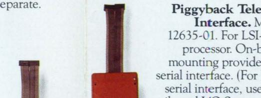
**Piggyback Teletype Interface.** Model 12635-01. For LSI-3/05 processor. On-board mounting provides bit-serial interface. (For byte-serial interface, use Distributed I/O System with Current-Loop Serial Intelligent Cable.)
