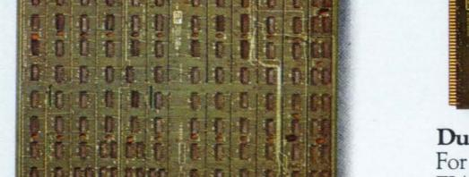
**Dual CRT Interface.** Model 14236-1X. For two CRT's or leased line modems. EIA RS232 interface with two half-duplex channels, each with one output control line and one input status line. Baud rates from 110 to 9600.
