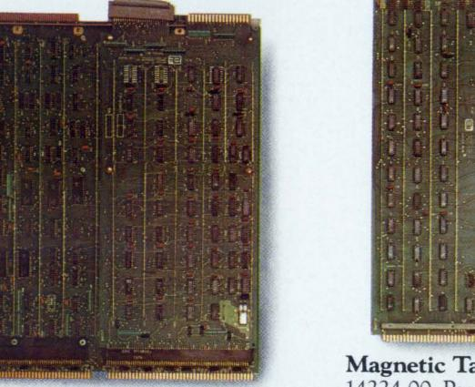
**NAKED MINI LSI-2/20 CPU.** Model 10400-00. Designed for high-performance applications. Twice the performance of the LSI-2/10 for only a nominal increase in cost. Also includes Power Fail Restart.
