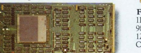
**Half-card Core Memory.** Model 11671-XX. 4K words. For either NAKED MILLI/ALPHA LSI-3/05 or NAKED MINI/ALPHA LSI-2 Series Computers.
