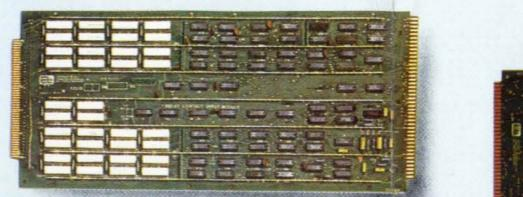
**32-bit Relay Output Module.** Model 13214-20. Operates as one 32-bit, two 16-bit, or four 8-bit outputs.
