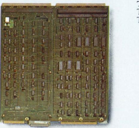
**NAKED MINI LSI-2/10 CPU.** Model 10600-00. 16-bit minicomputer processor offers twice the speed of LSI-3/05 processors. Includes Power Fail Restart option. See ALPHA LSI-2/10
