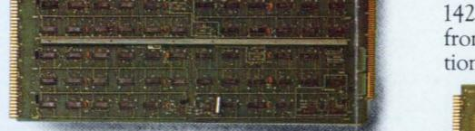
**Automatic Calling Unit (ACU) Multiplexer.** Model 13523-0X. Provides interfaces for one to four Model 801 ACU's, or equivalent. Simultaneous operations, full digit buffering and sense date-line busy. Four vectored interrupts per ACU. Available for either two or four ACU's.
