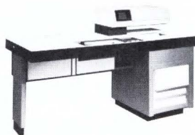
1790 Logic-Circuit Analyzer A basic functional and diagnostic test system for logic elements.
